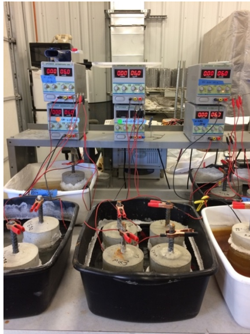
Figure 2. 8: Accelerated Corrosion Setup
