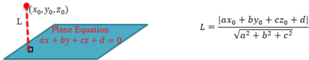
Figure 6 Equations used to calculate the height of a given point on a vehicle to the roadway surface represented by a plane
