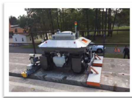
FHWA's RABIT Bridge Deck Assessment Tool rapidly detects and documents rebar corrosion, delamination, and concrete degradation.
