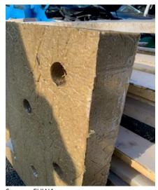
Source: FHWA A closeup view of one of the experimental polymer concrete segments.
