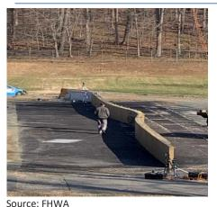
A man walks in front of a portion of the barrier that was moved by the test vehicle during the crash test at the FOIL.
