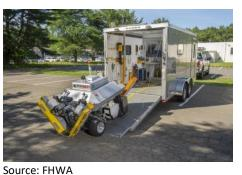
RABIT<sup>™</sup> being deployed from the systems operations center. The center is used to store and transport the equipment.
