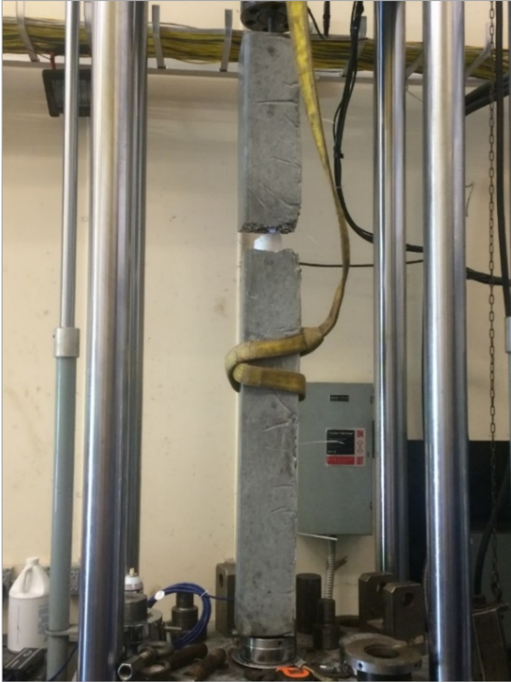
Figure 2-6: Concrete specimen 1 fractured in tension
