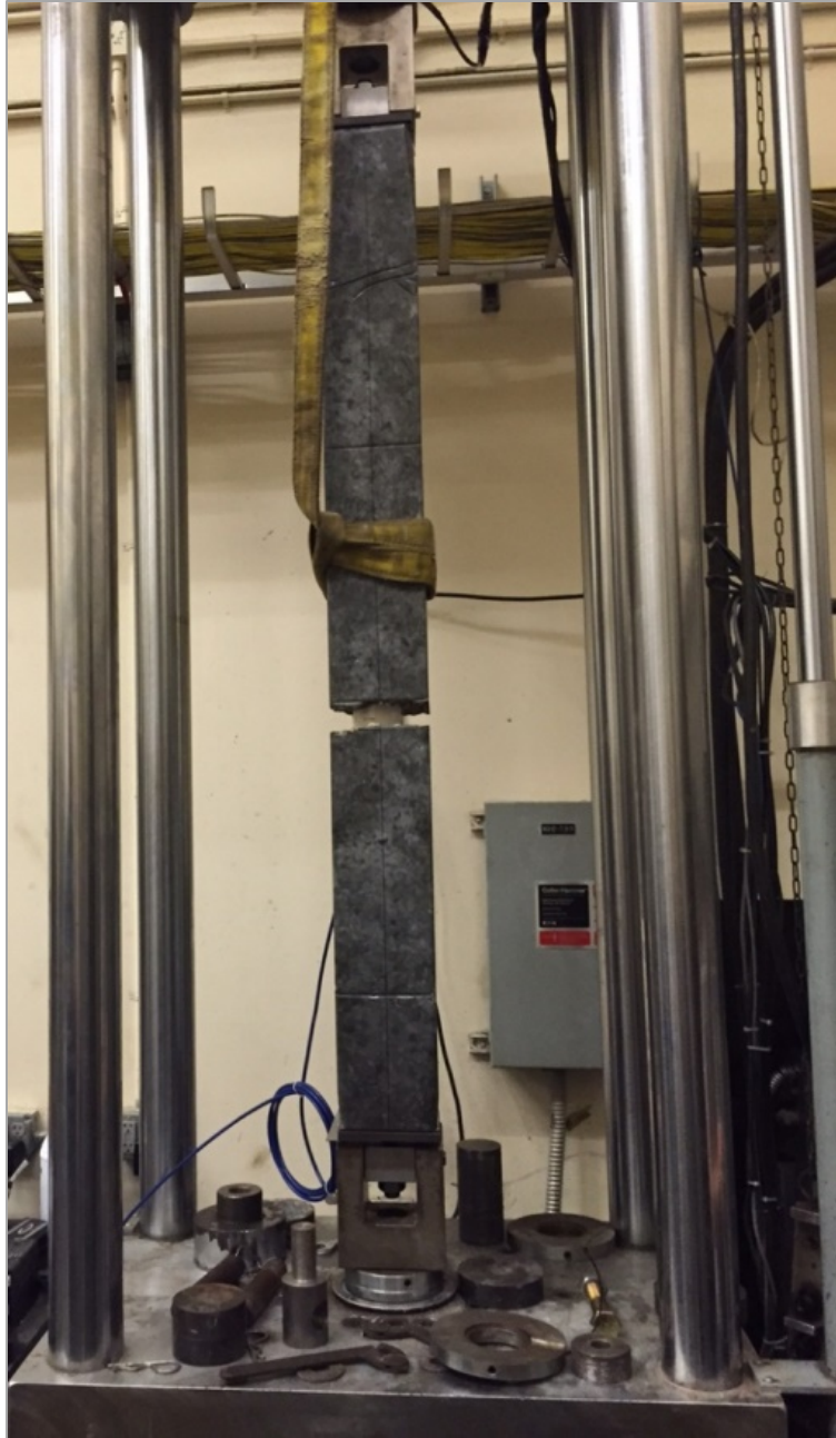
Figure 2-9: Testing of 6" x 6" x 60" concrete specimen 2 in tension
