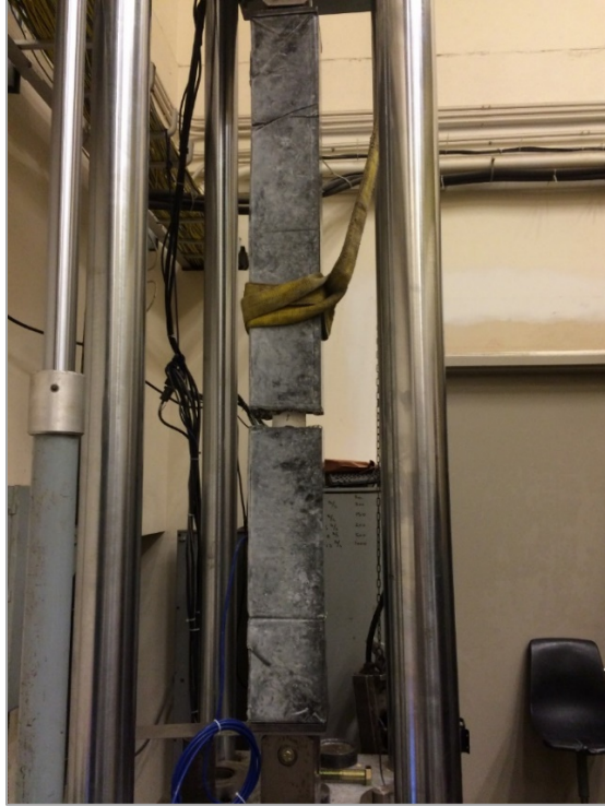
Figure 2-17: Specimen 2 failure in tension
