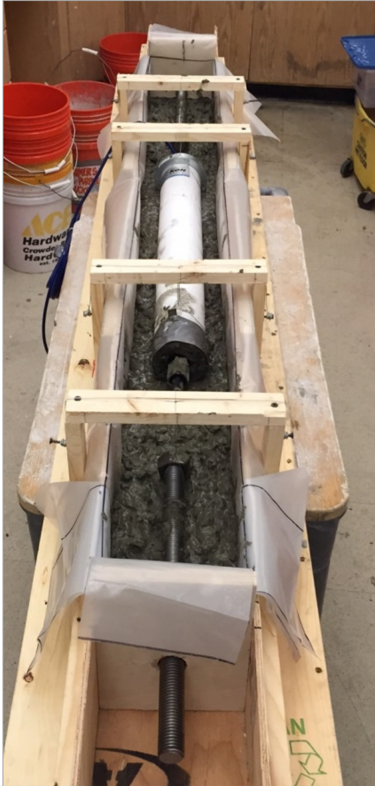
Figure 2-4: Concrete specimen fabrication
