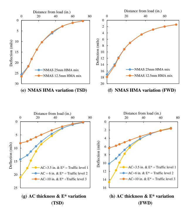
Figure 20 3D-Move output for varying pavement conditions
