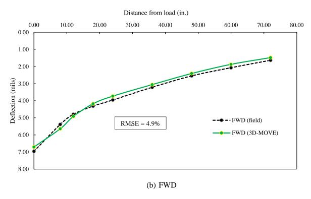
Figure 27 3D-Move generated deflection bowl validation on section 326-01 (LA 594-1)
