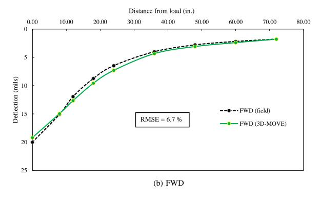
Figure 28 3D-Move generated deflection bowl validation on section 333-03 (LA 582)
