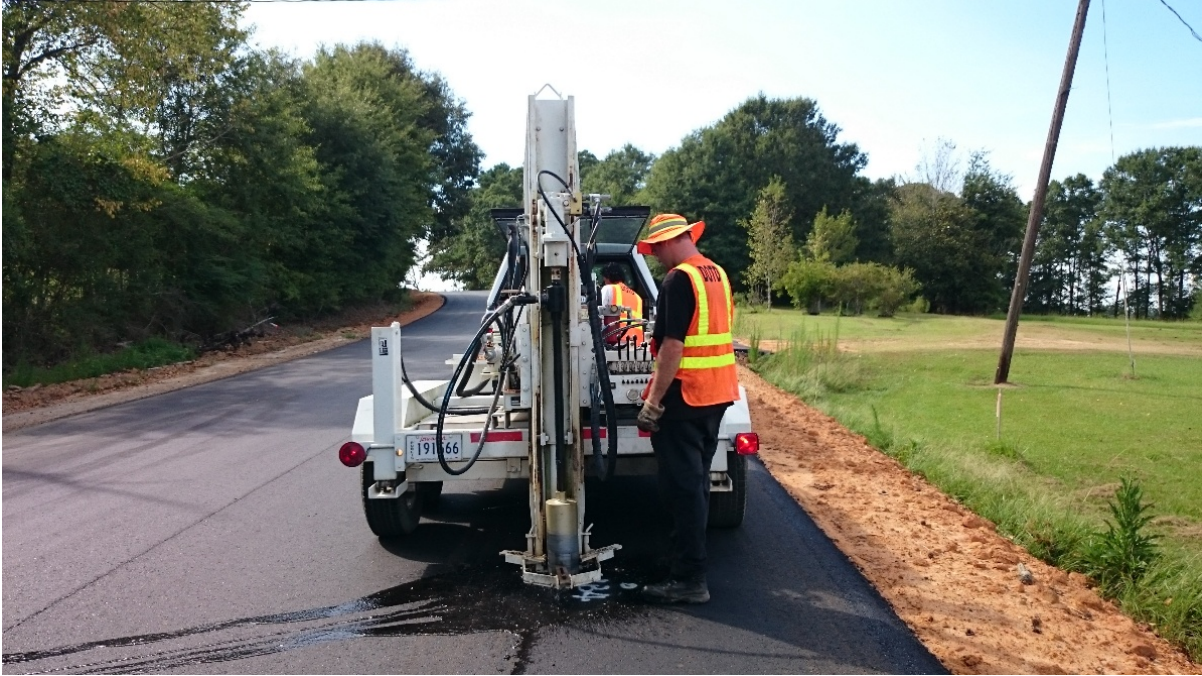
Figure 7 Field coring operation
