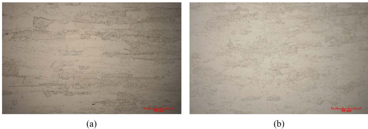
Figure 18. Micrographs From an ASTM A709 Grade 50CR Steel Plate Etched With Vilella's Reagent: (a) longitudinal sample at 1000X magnification; (b) transverse sample at 1000X magnification
