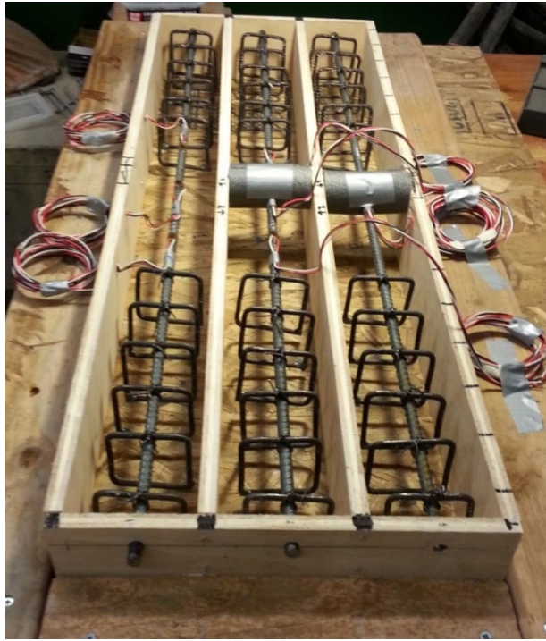
Figure 2.3 Small-scale beam forms with foam cylinders for access holes
