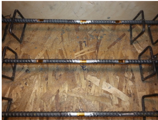
Figure 2.6 Strain gage layout
