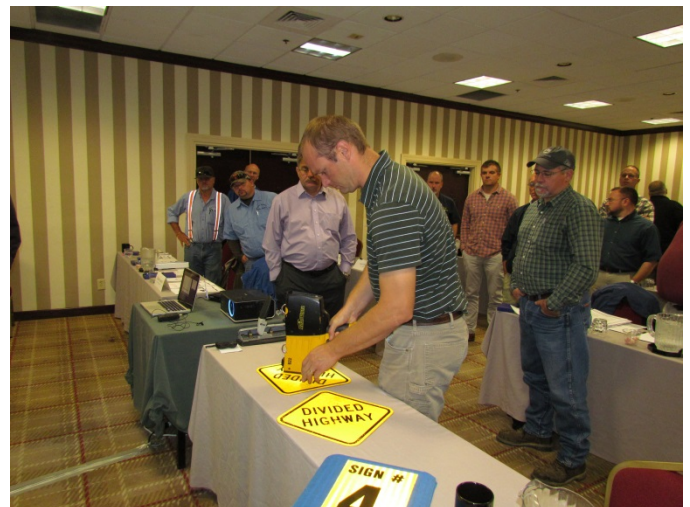
Luke Mantle, Road Supervisor with the Campbell County Road Department, tests a sign using the retroreflectometer.
