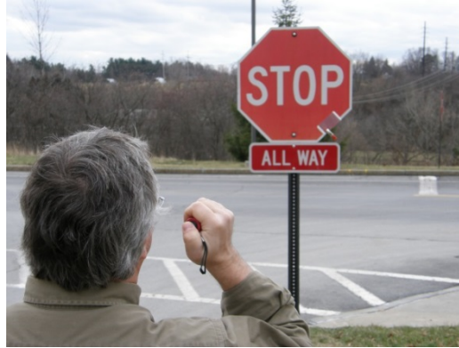
After attaching an inspection panel from CLRP's inspection kit to a sign, a simple hand-held flashlight is used to inspect a sign's retroreflectivity against the inspection panel (actual inspections are performed at night).
