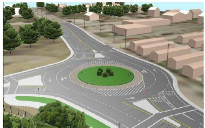
3-D design rendering used during an RSA in Rhode Island (Source: FHWA).
