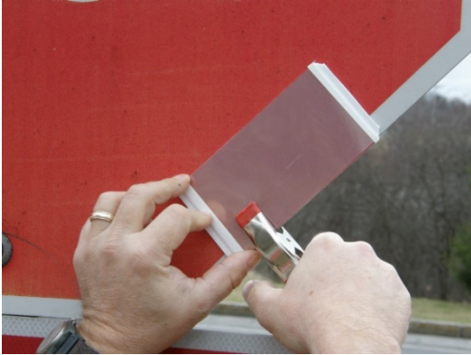
After attaching an inspection panel from CLRP's inspection kit to a sign, a simple hand-held flashlight is used to inspect a sign's retroreflectivity against the inspection panel (actual inspections are performed at night).
