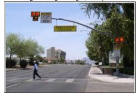
The alternating flashing red phase allows the delay to traffic to match the actual crossing needs of the pedestrians. Drivers can proceed with a stop-and-go operation during the flashing red phase. If pedestrians need more time, then the drivers remain stopped until they finish crossing. The ability to balance the pedestrian needs with driver delay is a valuable component of the HAWK treatment.
