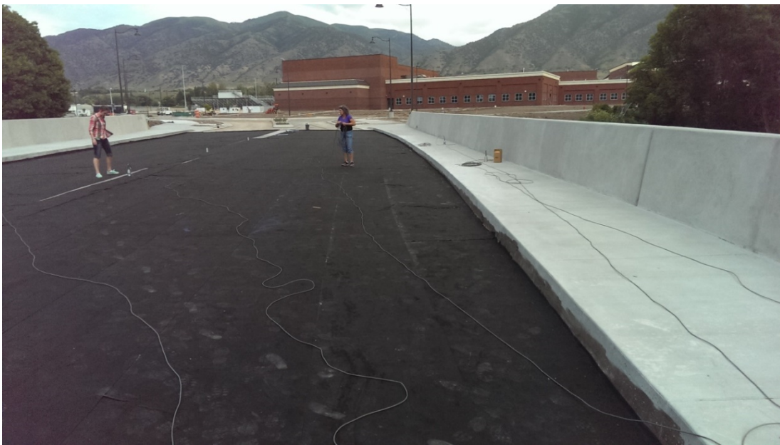
Figure 3.1: Preparing Sensors for the Impact Test
