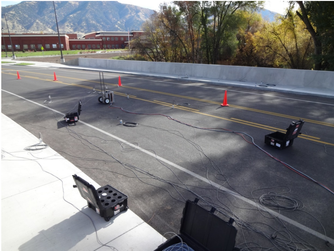
Figure 3.10: Sensors and the Shaker during the Second Shaker Test
