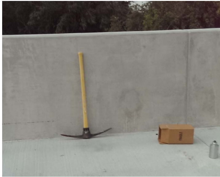
Figure 3.2: Pickaxe used to Excite the Bridge during Impact Test
