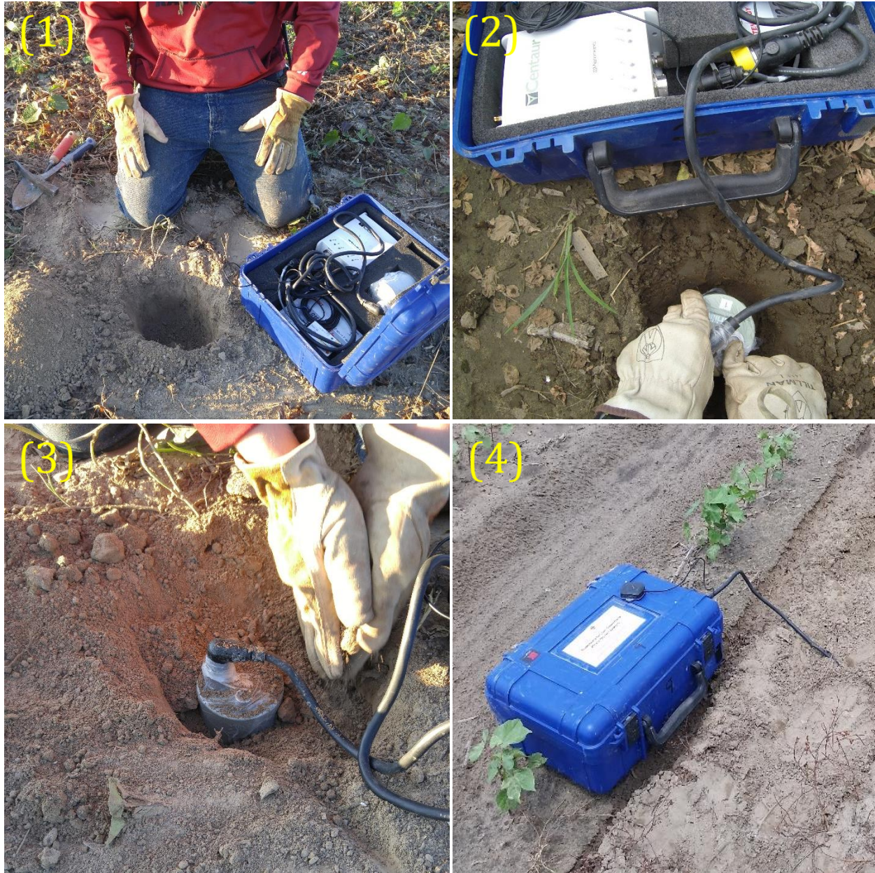
Figure 2. 10: (1) A 15 centimeter diameter hole is dug to a depth of approximately 15-30 centimeters. (2) A Trillium Compact seismometer is placed in the hole, oriented toward magnetic North, and leveled. (3) The soil is replaced around the sensor and compacted to ensure sufficient coupling. (4) The station is allowed to record data for 1-2 hours.
