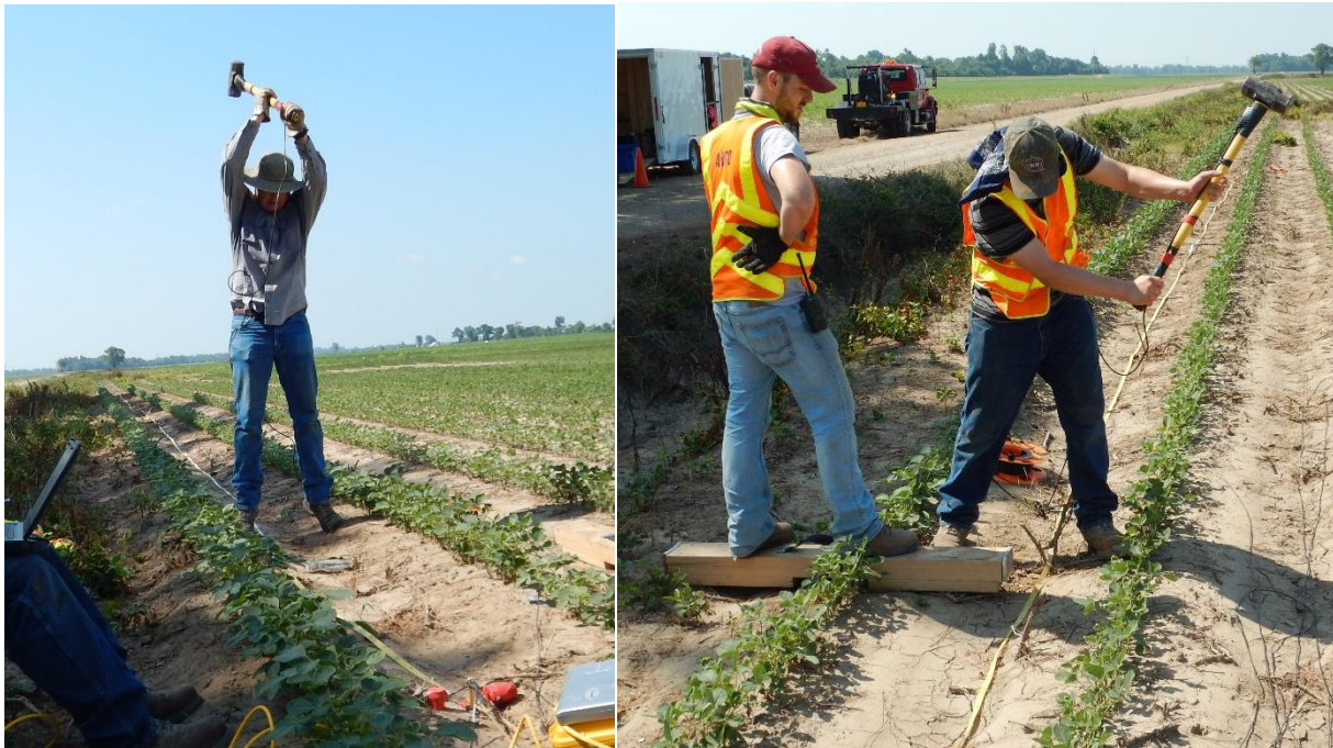
Figure 2. 5: Left - A sledgehammer impacted vertically being used to generate Rayleigh waves. Right - A sledgehammer impacted horizontally being used to generated Love waves.
