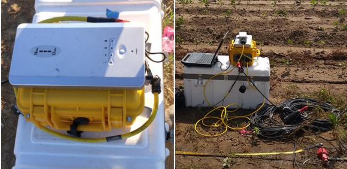
Figure 2. 4: Left - A Geometrics Geode Seismograph with portable battery attached to the top. Right: A geode linking the geophone refraction cable and field laptop.
