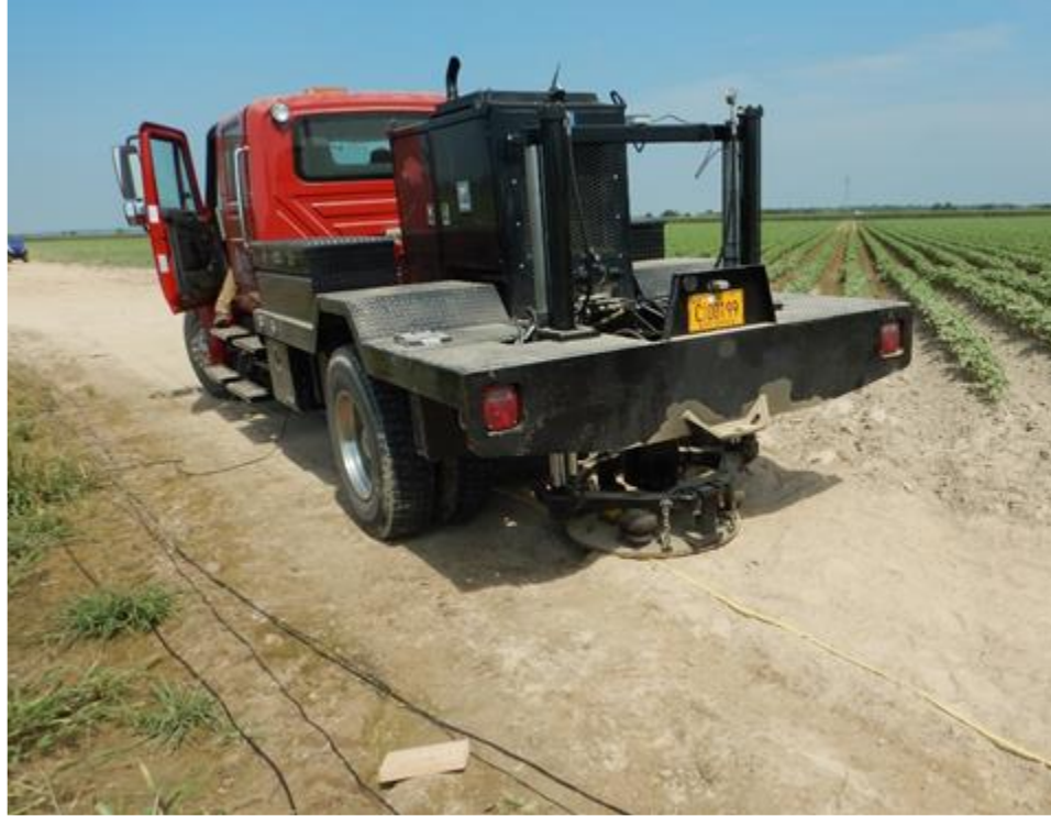
Figure 2. 6: A vibroseis truck being used as a source of excitation for surface wave testing.
