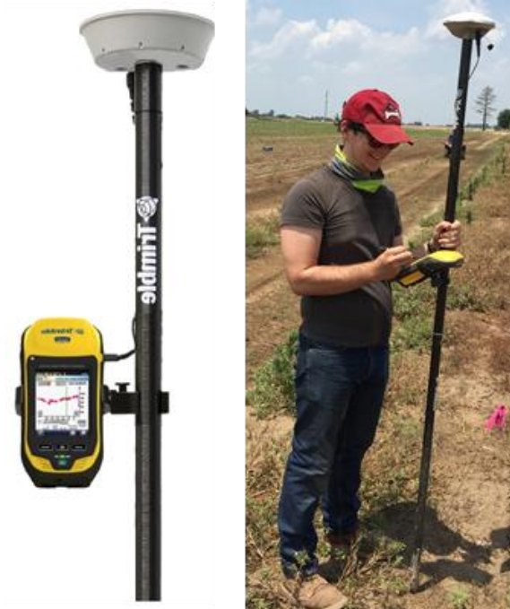
Figure 2. 11: Trimble GPS with external antenna.
