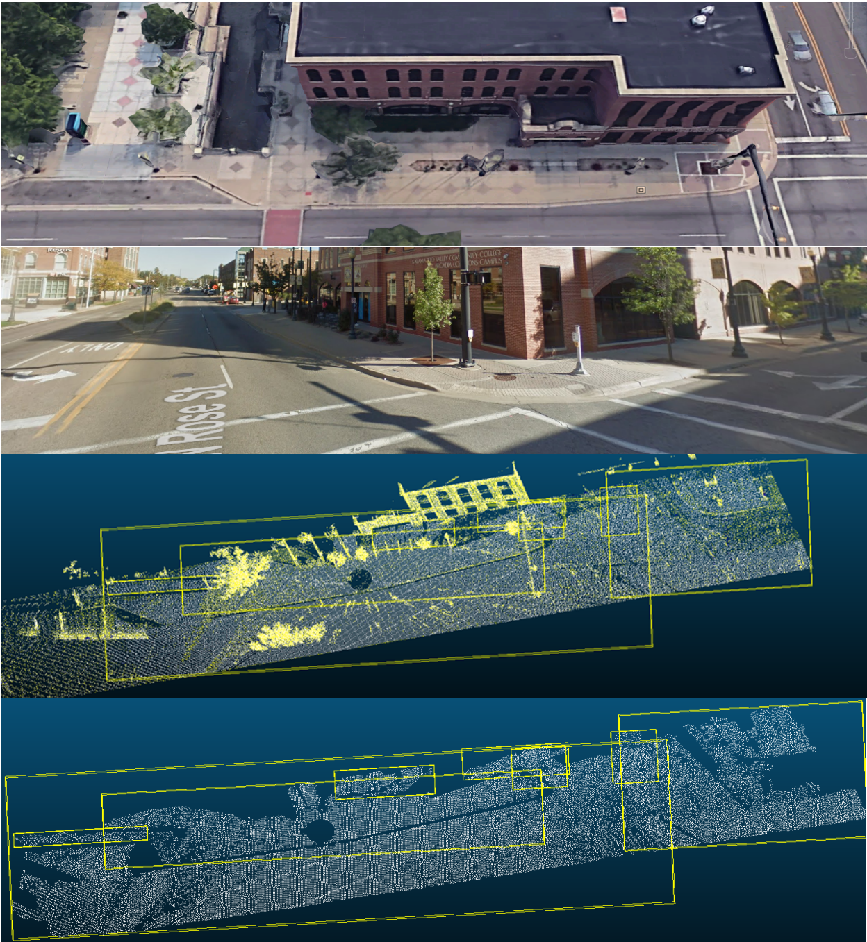
Figure 12: Sidewalk and ramp detection flow in automated PCD (top view, front view, full top PCD view, surface top PCD view)
