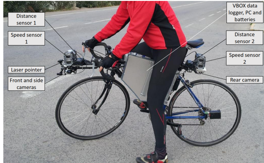
Figure 2-1: The instrumented bicycle used in Llorca's study (Llorca et al., 2017)
