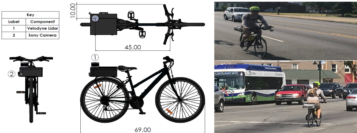
Figure 3-11: Lidar and bicycle set up
