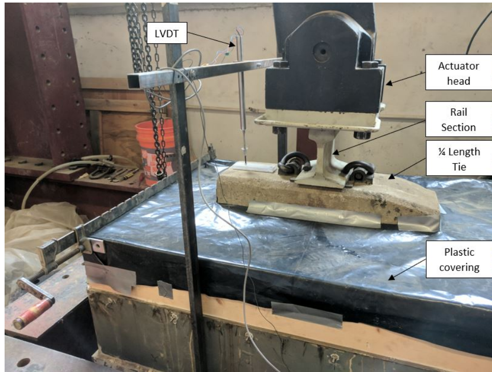
Figure 4 – Completed box test setup showing LVDT placement and plastic covering to prevent moisture loss
