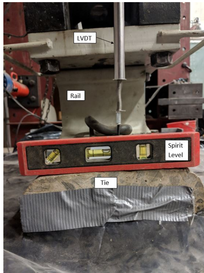
Figure 12 – Tie rotation after failure in the 30 percent fouled box test with abraded ballast and natural fouling
