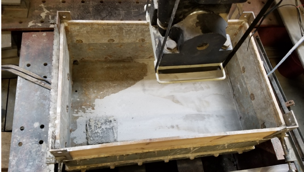
Figure 3 – Top-down view of the empty box in the frame with wooden boards attached
