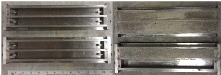
Fig. 3.3.1-1 Mortar-Bar mold with gage studs (left) and mortar-bar mold with three mortar-bars (right).
