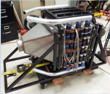
Figure 23 Thermoelectric Generator (TEG) Designed and Built for Transit Diesel Buses
