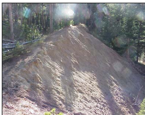
Abandoned tailings piles can be a source of metal contamination to waterways.
