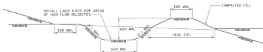
TYPICAL DRAINAGE SWALE
