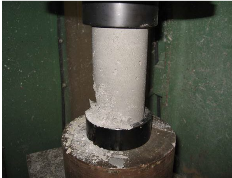
Figure 5 Phoscrete compression test 1 hour after mixing at 0 °F
