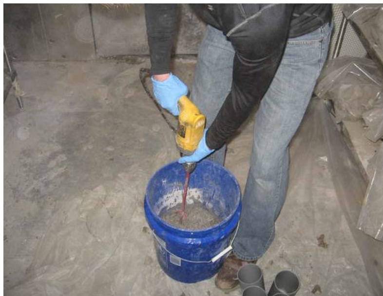
Figure 3 Mixing of MG-Krete at 35 °F for Cylinder Preparation
