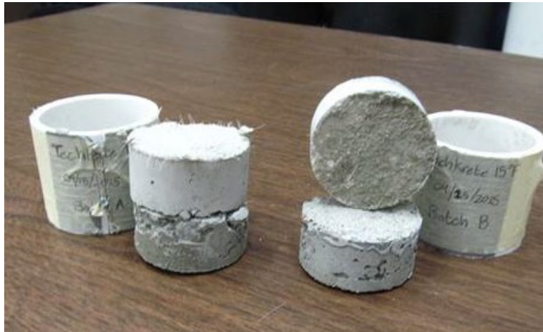
Figure 7 Tekrete Bond Shear Specimens After Failure
