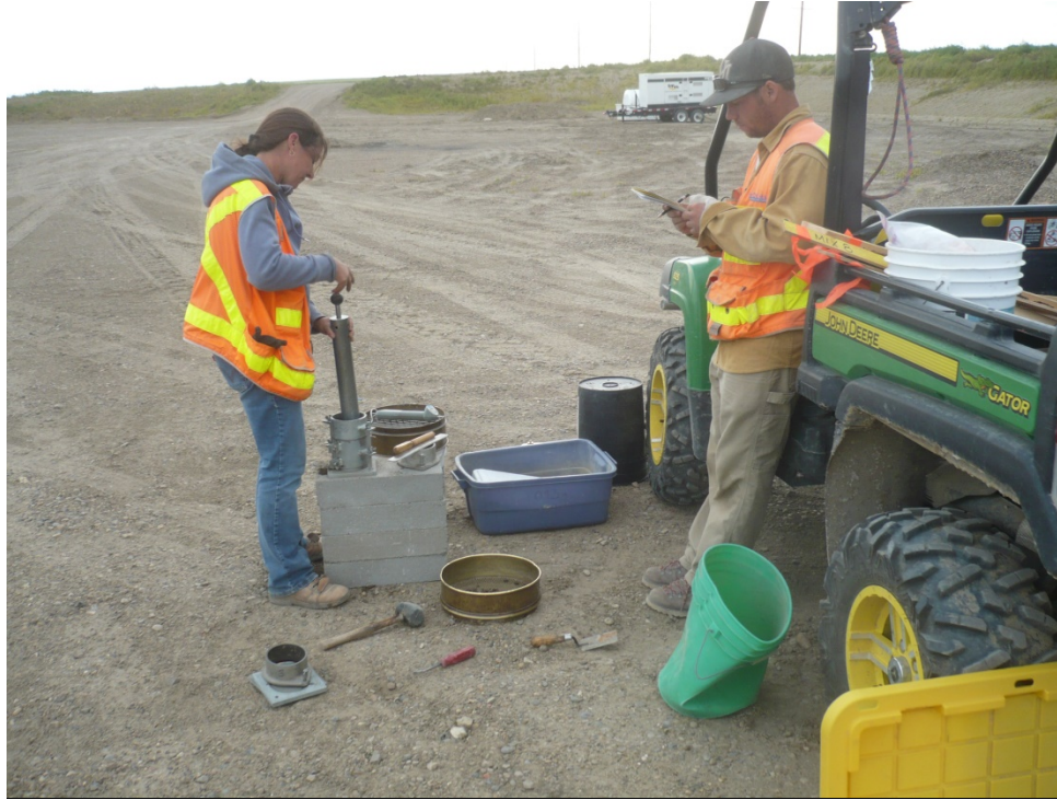
FIG. 29. Single point proctor sample pounded on site immediately after sampling.
