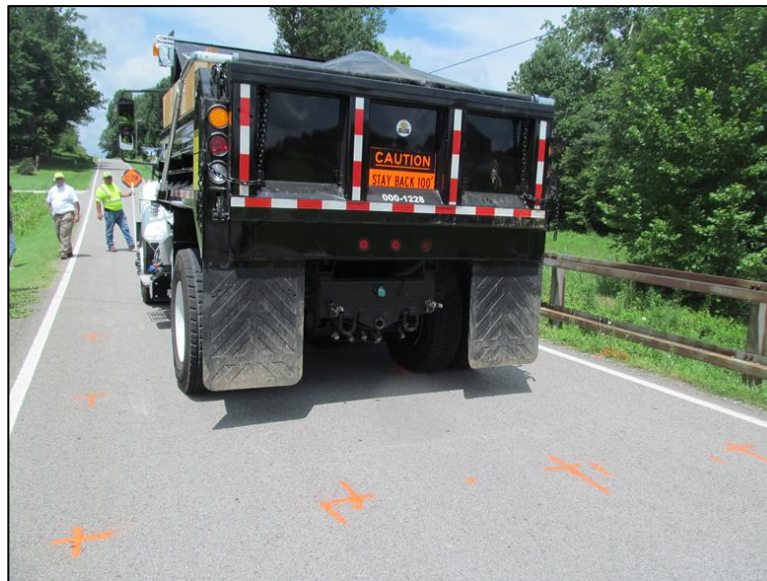
Fig. 21 Positioning of load test truck on bridge deck
