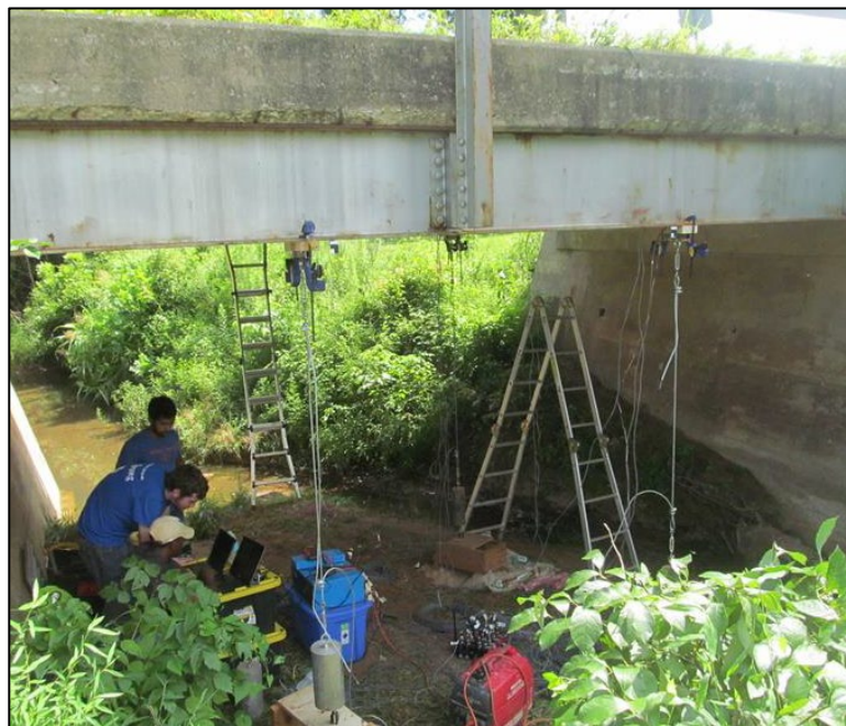
Fig. 20 Layout of data acquisition systems underneath the bridge
