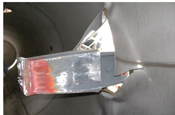
Figure 6. Post-test Tear in Inner Tank
