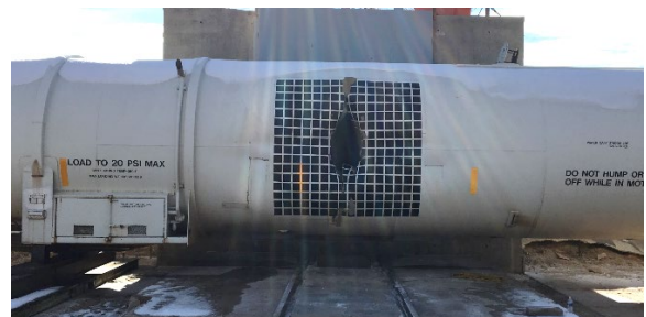
Figure 2. Post-test Photo of the Punctured Shell
