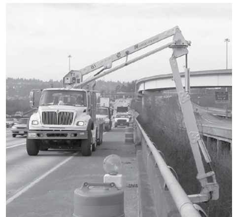
Top right: A visual inspection of a steel girder bridge is conducted. Middle right: An inspector conducts a visual inspection of a truss structure. Bottom right: An under-bridge inspection vehicle is used on an Interstate bridge. Bottom left: A visual inspection is carried out for a steel substructure unit.
