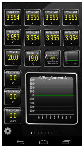
Figure 77: Prototype wireless diagnostics using an off-the-shelf app and wireless connector (Chevrolet Volt data shown)
