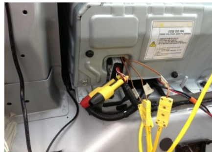
Figure 48: Direct BMS communication access (Hyundai Sonata Hybrid)
