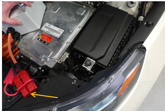
Figure 59: Developed prototype connector for high-voltage terminal access
