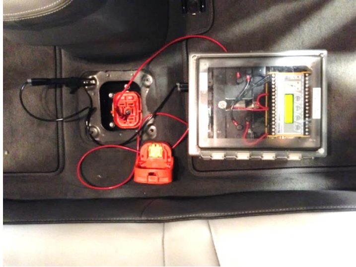
Figure 79: Tool installation in a BEV to evaluate isolation of half pack via removed MSD
