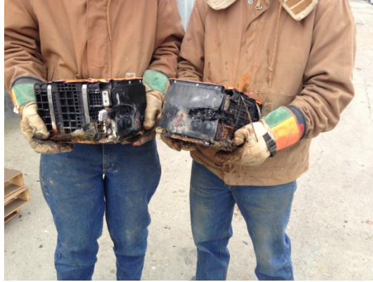
Figure 23: Module enclosure damage
