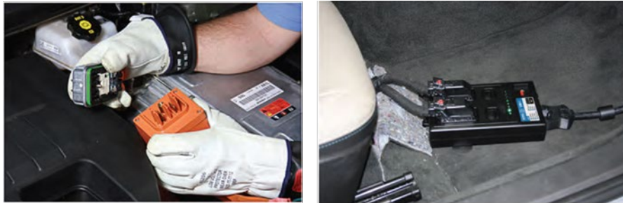
Figure 13: GRX-5100 example connectors and adaptors [4]
