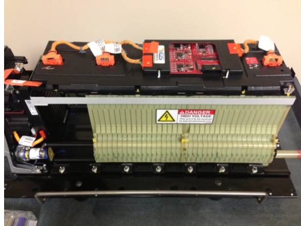
Figure 5: Chevrolet Volt Battery Module and BMS sub-system
