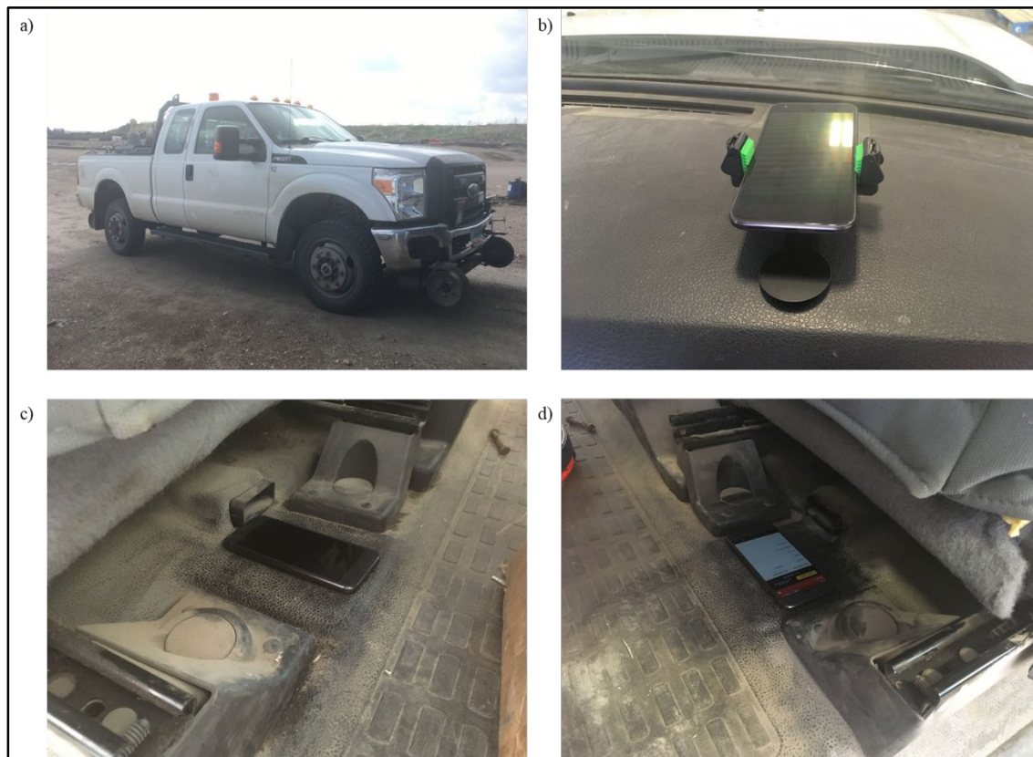
Figure 4.2 a) HY-RAIL® vehicle used; b) Phone 1 installed on dashboard; c) Phone 2 installed under driver seat; d) Phone 3 installed under passenger seat
