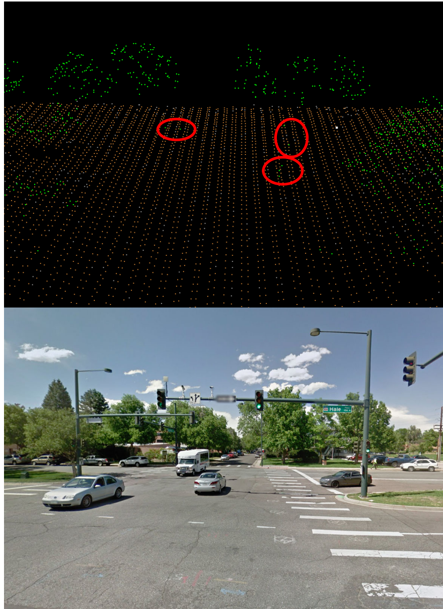
Figure 11.1 QL2 Data of Street Intersection; Street Light and Traffic Light Features are Circled in the Top LiDAR Point-Cloud
