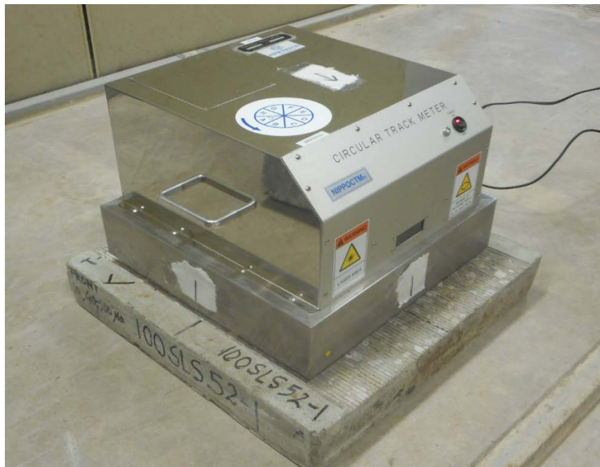
Figure 3-12. Circular track meter (CTM) setup on a ground slab specimen.
