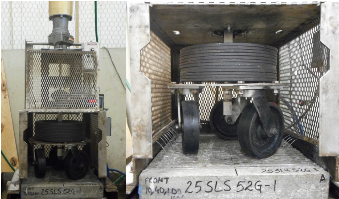
Figure 3-7. Three wheel polishing device (TWP) developed by NCAT which was used for this study. The NCAT version was modified as described in (Whitney et al. 2013).
