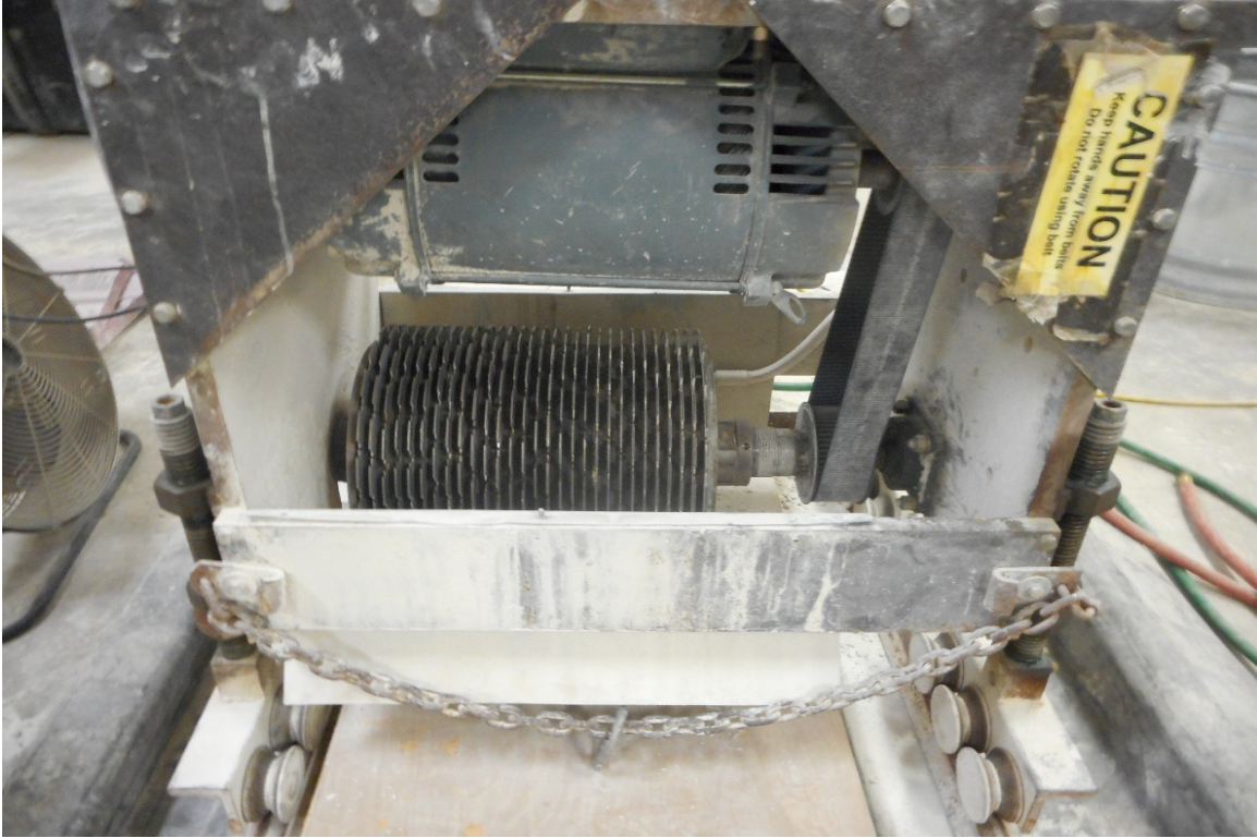
Figure 3-4. Grinding machine used to apply texture to slab specimens. Shown with a fully stacked shaft.
