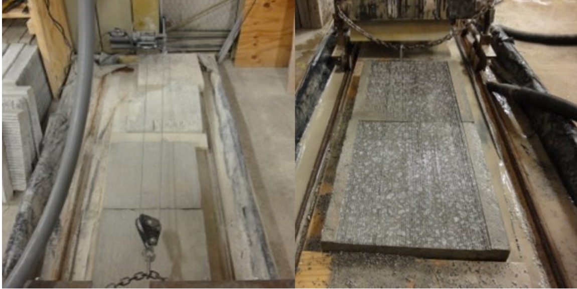
Figure 3-6. Before and after images of texture application process. The image on the left shows slabs with as-is texture and the image on the right shows slabs with the applied texture.
