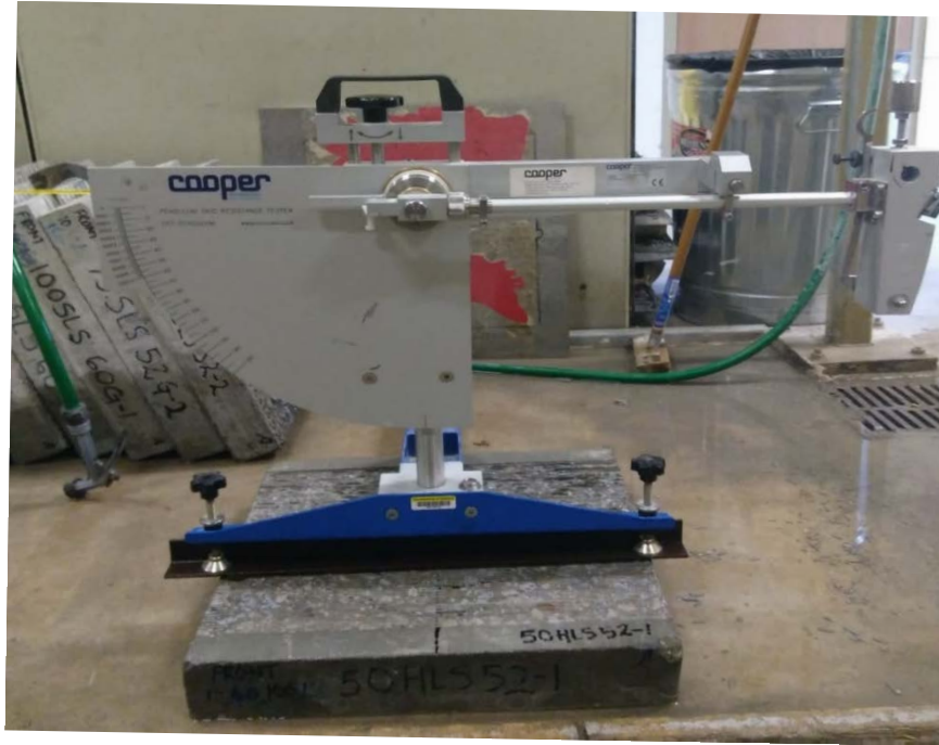
Figure 3-9. British pendulum tester (BPT) setup on a ground and polished slab specimen.
