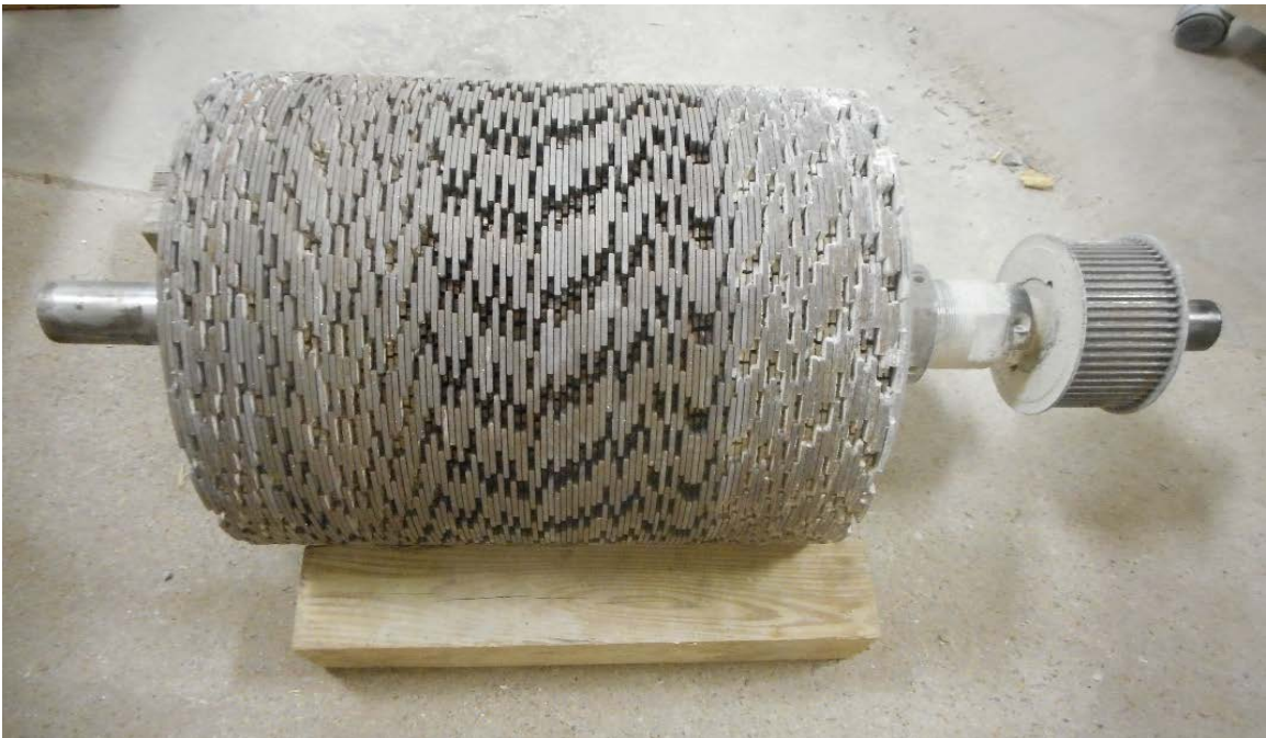
Figure 3-5. Fully stacked shaft close-up with blades and spacers.
