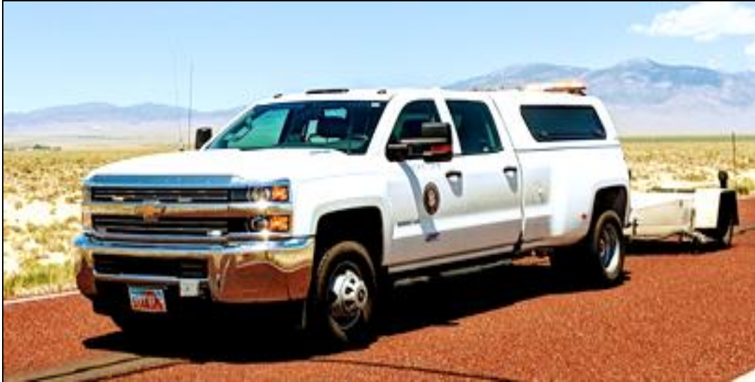
Figure 3.1 UDOT Skid Data Collection Truck and Trailer
