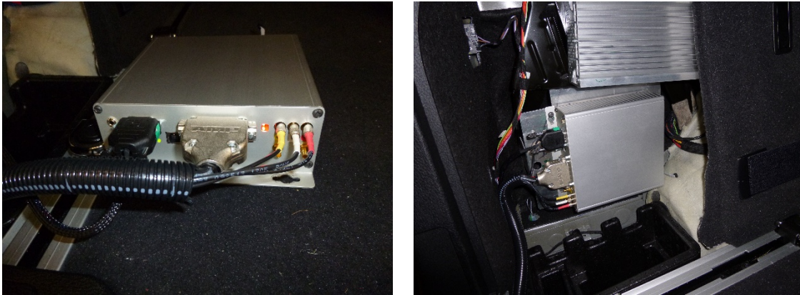
Figure 2. Data Acquisition System Enclosure.
