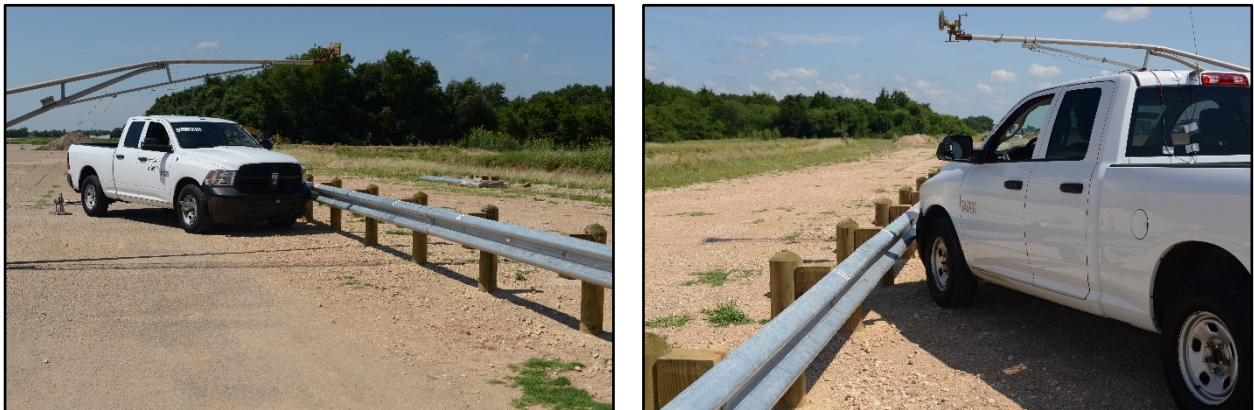
Figure 5.1. Guardrail/Test Vehicle Geometrics for Test No. 469688-5-1.
