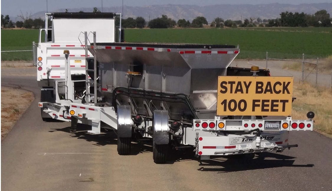
Figure 3: TowPlow2 – Option-3 Sander Configuration
