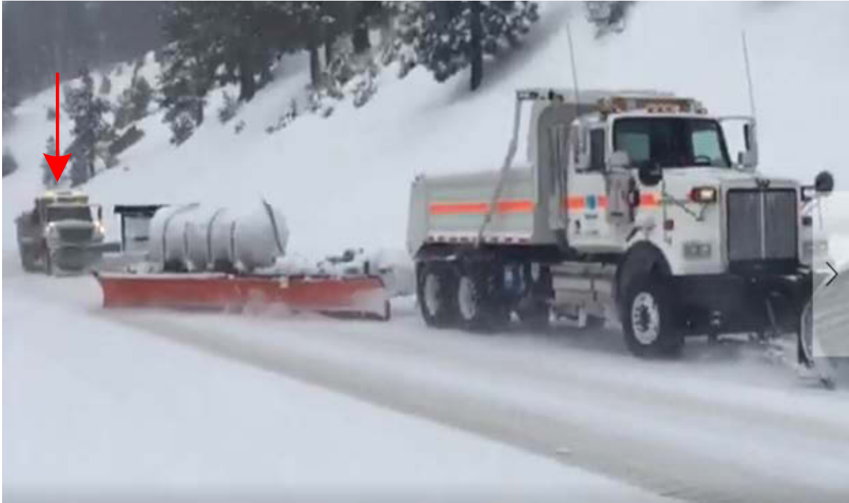
Figure 17: Additional Sander Truck Trailing TP2-DoE on I-80
