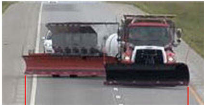
Two Lanes of Clearing with 12-ft Head Plow
