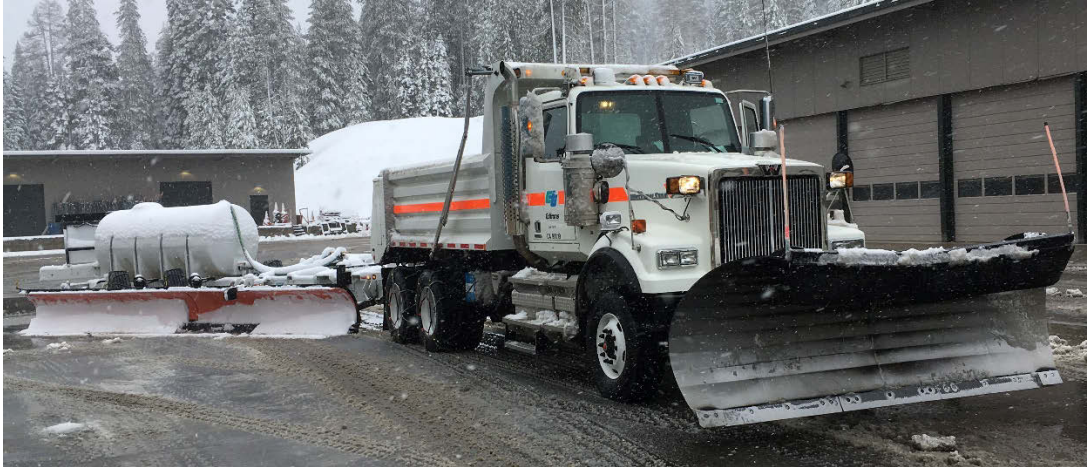
Figure 11: TowPlow with 22-Foot Snow Clearing Path
