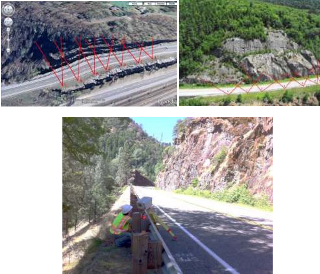
Figure 71. Top left, a) Scanning from the highway median at the New York site; top right, b) Scanning from the highway median at the New Hampshire site; and bottom, c) Difficult scanning from across a narrow highway at the California site.
