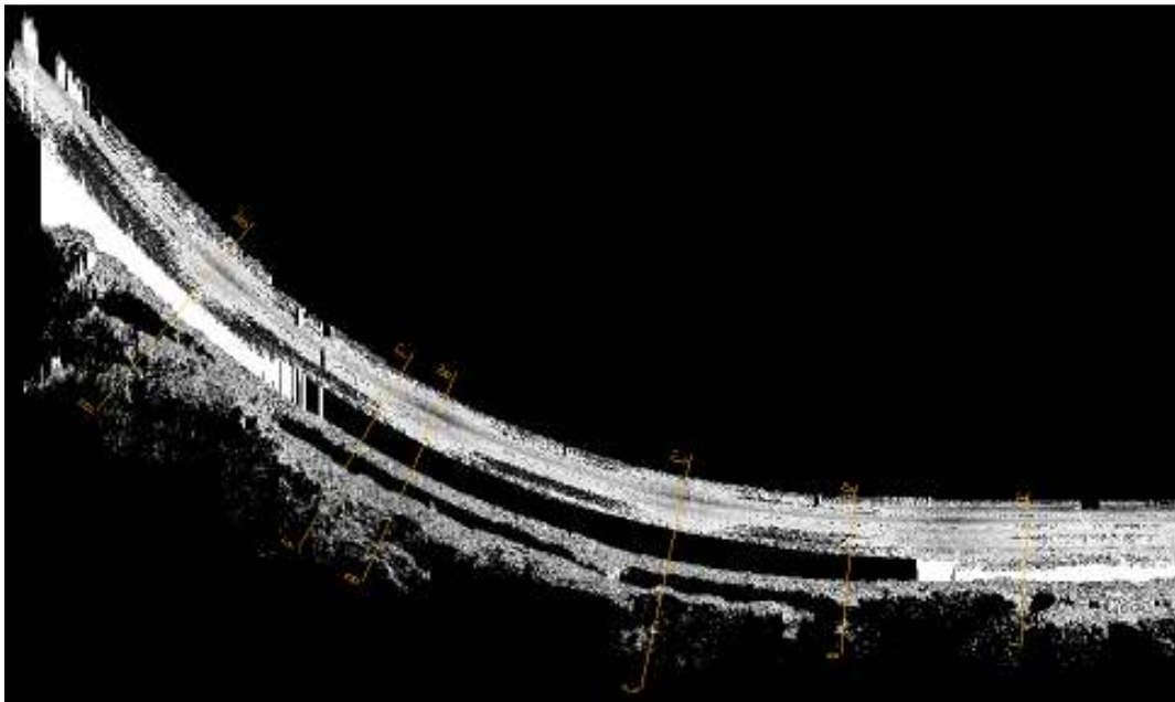
Figure 60. Aerial view (z direction) of I-24 with lanes scan, showing Sections A–F.
