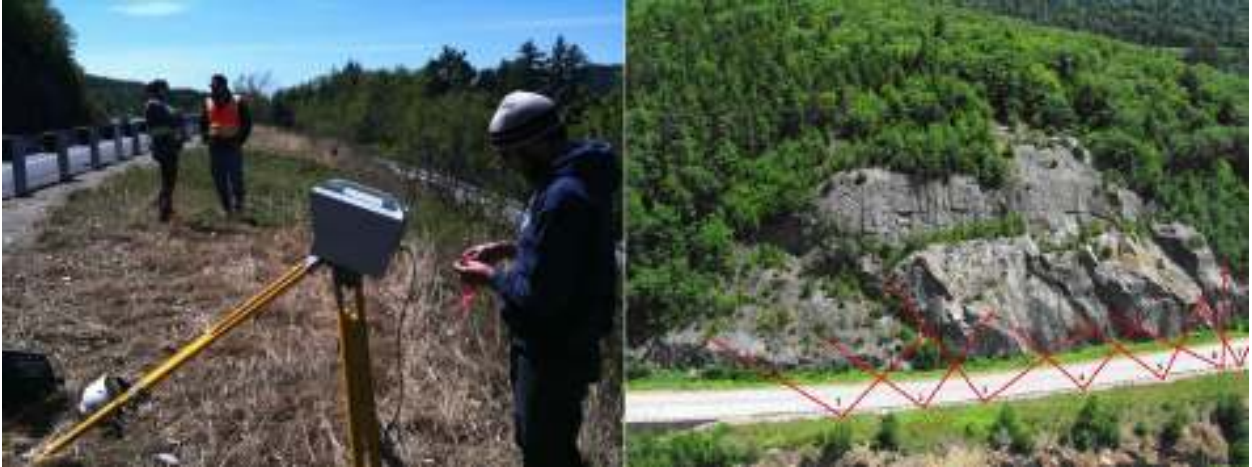
Figure 32. Left to right, an example of scanning at the site using an Optech ILRIS 3D scanner, and the approximate locations of scans Woodstock1 to Woodstock7.
