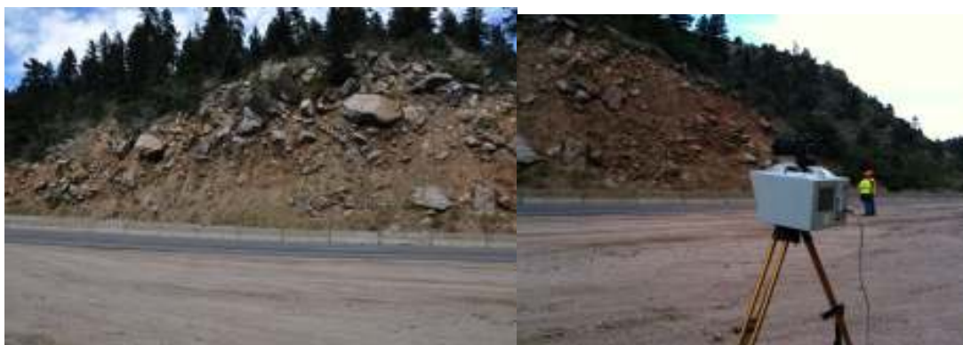
Figure 25. Colorado Site 1 along with the scanner used, an Optech ILRIS3D.
