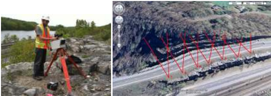
Figure 40. Left to right, an example of scanning at the site using an Optech ILRIS 3D scanner, and the approximate locations of scans Mohawk1 to Mohawk7.
