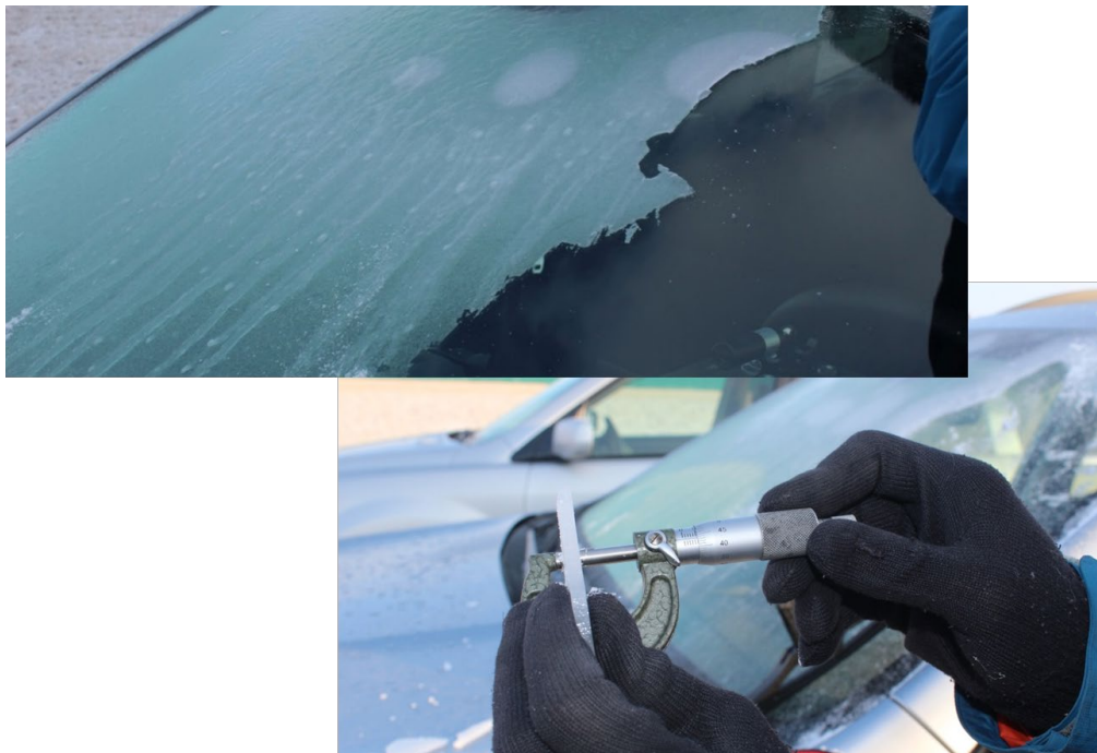
Figure 10. Photos. Sample of ice buildup achieved on test vehicles for testing.
