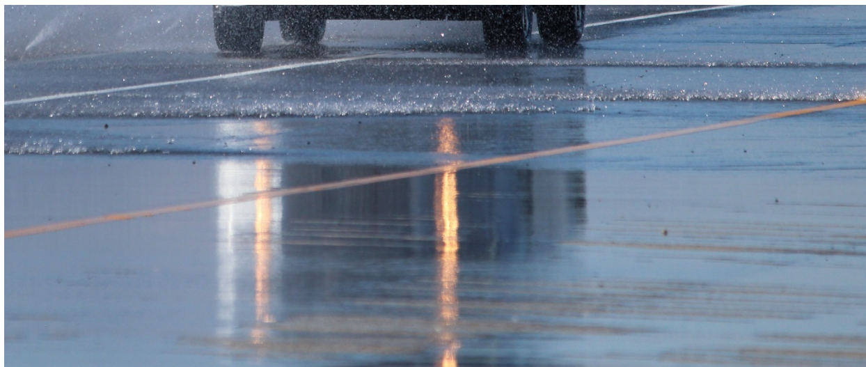
Figure 12. Photo. Wet road caused by water spray on the Winding Road Course.
