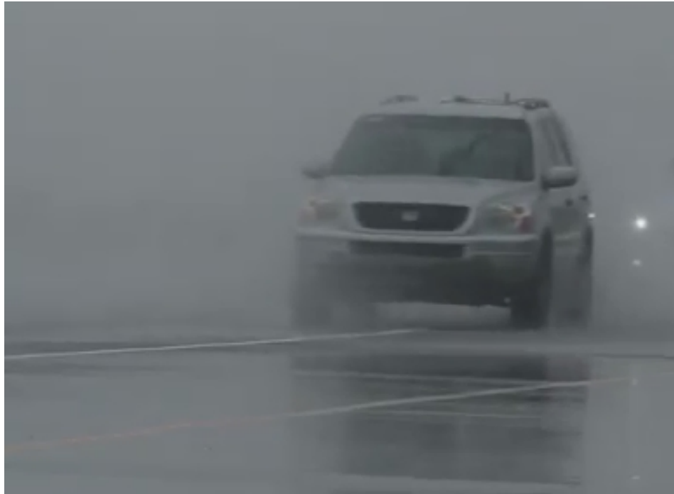
Figure 4. Photo. Water spraying in the vehicle path on the Winding Road Course as the principal other vehicle (POV) drives through.
