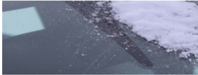
Figure 18. Snow applied to sensors on vehicle under test.
