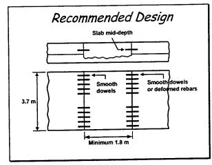
Full-depth repairs should be at least 1.8 m (6 ft) to ensure the extent of deterioration is addressed and to provide a more stable repair that exhibits more slab-like behavior. Smooth dowels should be placed at one or both ends; deformed tiebars can be placed at one end only. The dowels should be placed at middepth within the slab.
