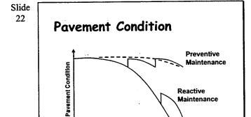
The difference between the effect of preventive and reactive maintenance is significant. Not only is the timing of application different, but the effect (represented by the slopes of the aftertreatment performance curves) is also different.
