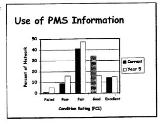
This figure illustrates an example of how pavement management data can be used to support preventive maintenance decisions very effectively. The example is from the City of Bedford, Texas.
