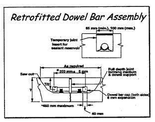
In the load transfer restoration process, slots are saw cut into the pavement. Dowels are placed on supports at mid-depth and backfilled with cementitious material and finished flush with existing pavement.
