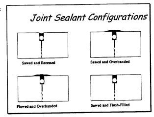
A variety of sealant placement configurations can be used. Sawed and recessed is the most commonly used configuration. Using this configuration, the existing joint is sawed to the desired width, the joint sidewalls are cleaned, a backer rod is installed, and the sealant material is placed with a slight recess below the surface.
