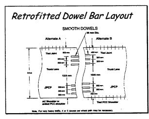
Dowels are generally clustered in groups of three dowels in each wheelpath. Groups of 4 or 5 dowels in each wheelpath may be required for very heavily-trafficked pavements.
