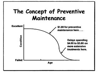
This chart illustrates why we can not afford to keep doing things the same old way. As the pavement first begins to deteriorate, the cost of repair is relatively inexpensive (like an oil change or tune up). However, as the progression deteriorates further, the costs increase exponentially (like an engine overhaul).
