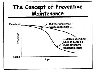
This chart illustrates why we can not afford to keep doing things the same old way. As the pavement first begins to deteriorate, the cost of repair is relatively inexpensive (like an oil change or tune up). However, as the progression deteriorates further, the costs increase exponentially (like an engine overhaul).
