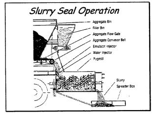
Specially designed equipment combines ingredients into a homogenous mixture and places the material on the pavement. The mixture is in the form of a creamy-textured slurry. Common fillers are portland cement, lime, and aluminum sulfate. Curing time is generally around 2 hours, although it can be as long as 12 hours, depending on the ambient temperature.
