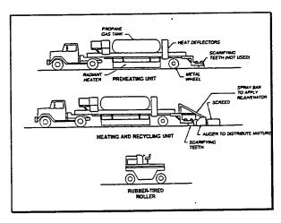
This is a schematic of the heater-scarification process. No new aggregate materials are added during this process, although a new wearing course is added later. Scarification depths typically are between 19 and 25 mm (0.75 and 1 in), although depths up to 50 mm (2 in) can be achieved.
