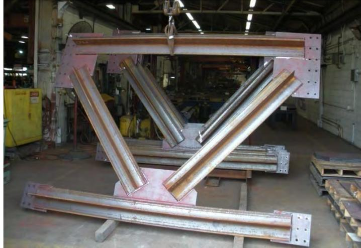
**Figure 6.6.3.5.3-1 Cross-Frame Composed of Structural Tees**
