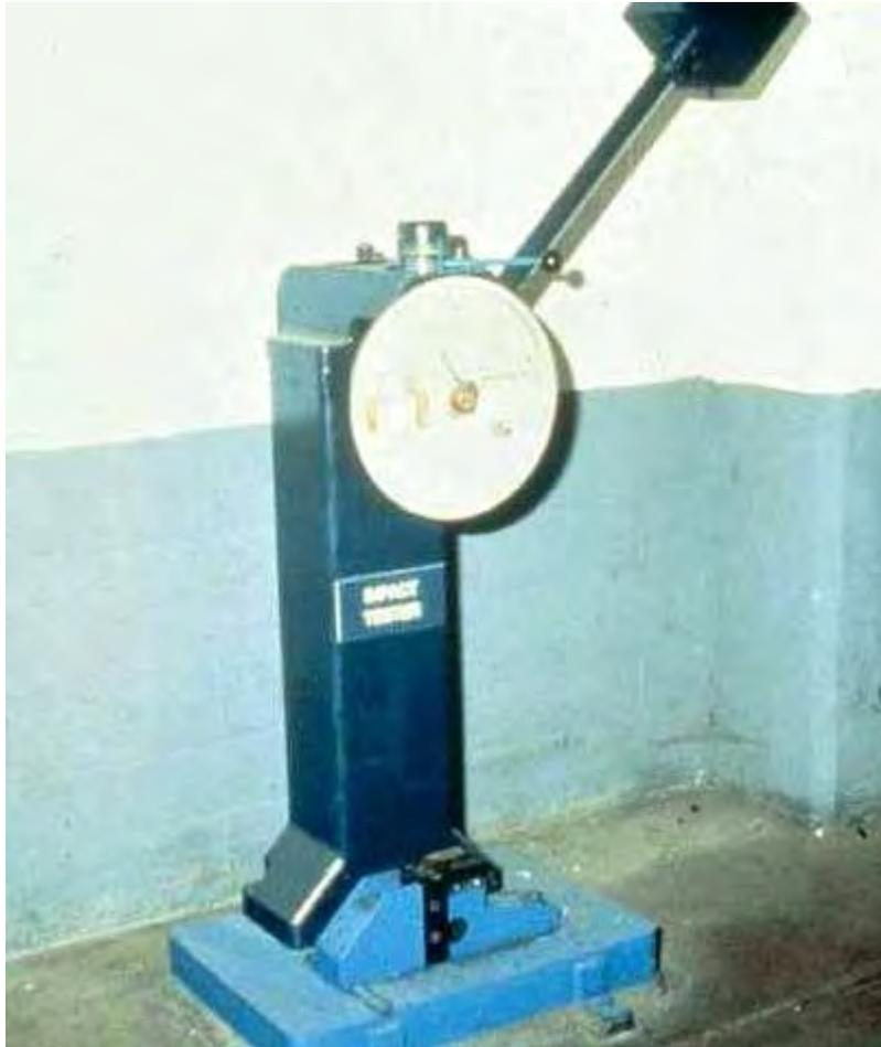
**Figure 6.5.5.3.2.1-1 Charpy V-Notch Testing Machine**
