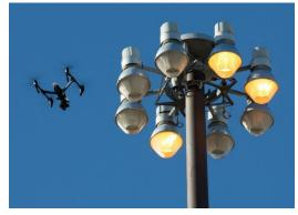
Figure 5: Image of a New Jersey DOT UAS inspecting a high mast light pole.
