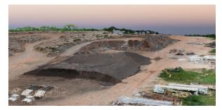
Figure 7: Image pulled from a Duit Construction video demonstrating using topographical imagery to assess material volumes in a recycle yard.
