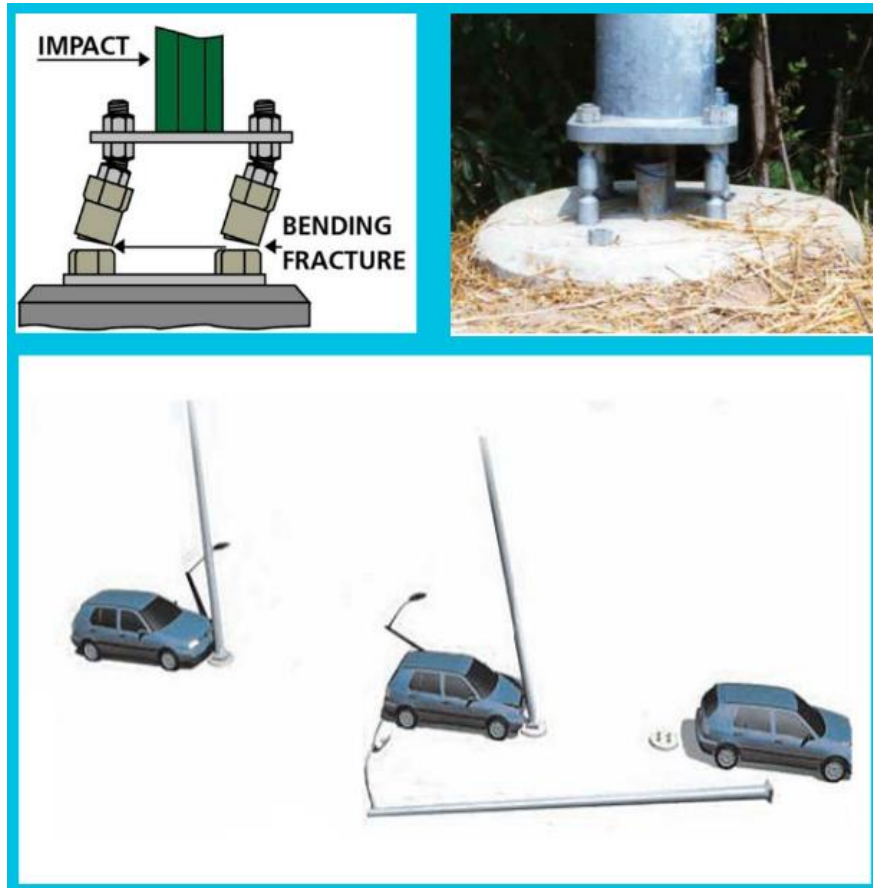
Top: Breakaway devices. Bottom: Example of what happens when a vehicle strikes a breakaway pole.
