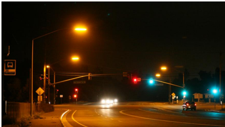
Appearance of a roadway under LPS streetlighting.
