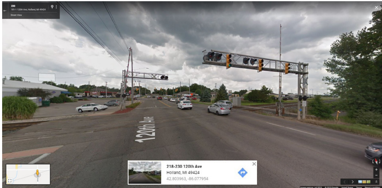
Figure 42. Illustrative Example of a Cantilever-Mounted Pre-Signal (CSX 120th Avenue Crossing at E. Lakewood Boulevard in Holland, MI, USDOT 234648C)
