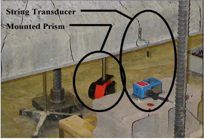
Figure 4.11. String Transducer and Mounted Target Prism
