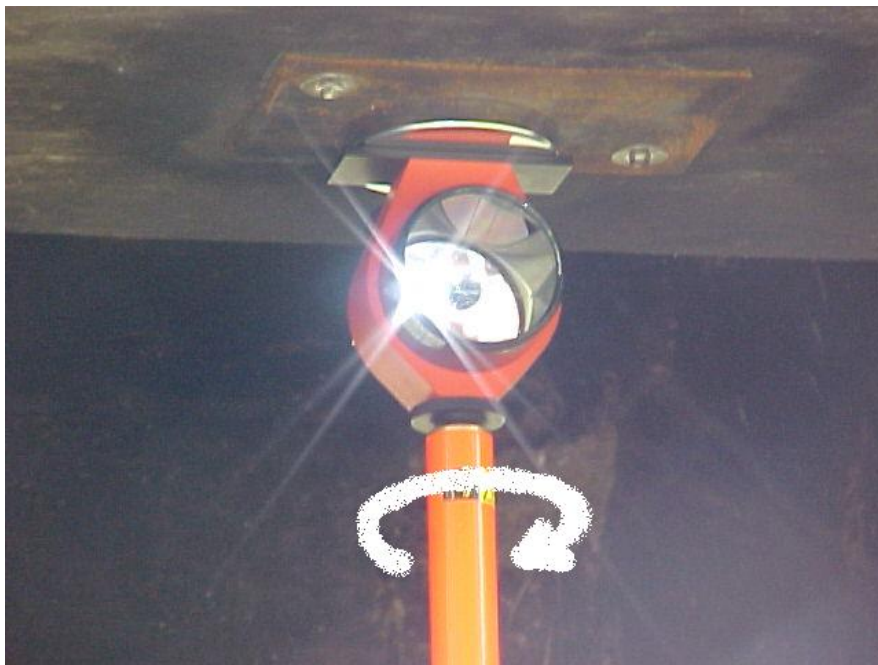
Figure C.5. Screw Range Pole onto Prism
