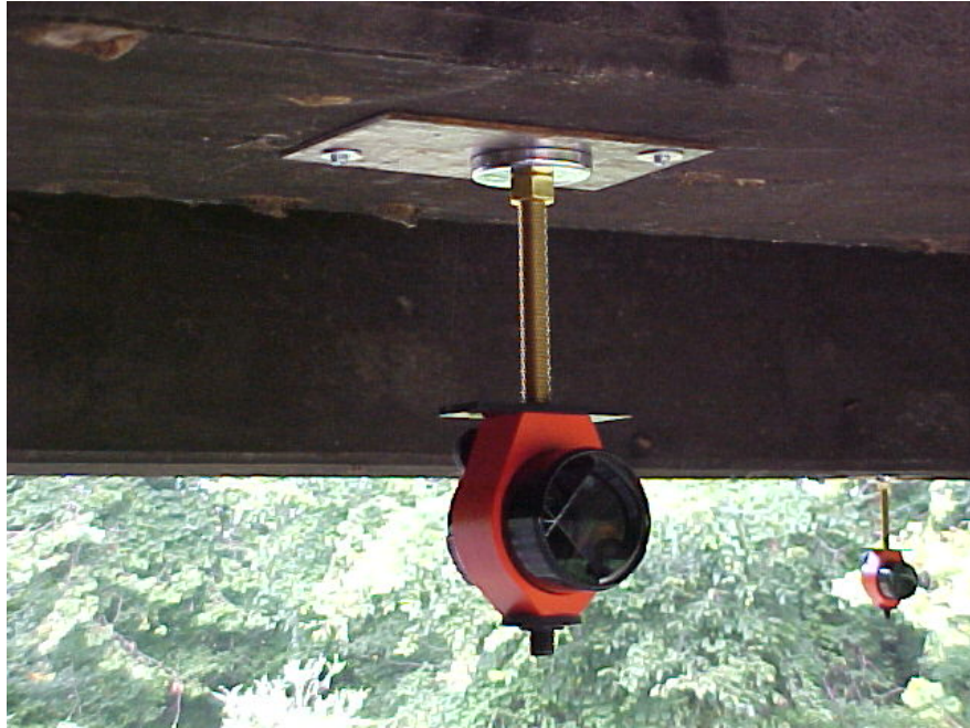
Figure C.4. Long Magnet Mount and Prism
