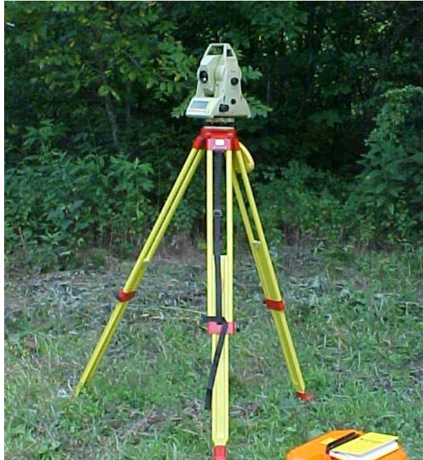
Figure C.1. Total Station and Tripod
