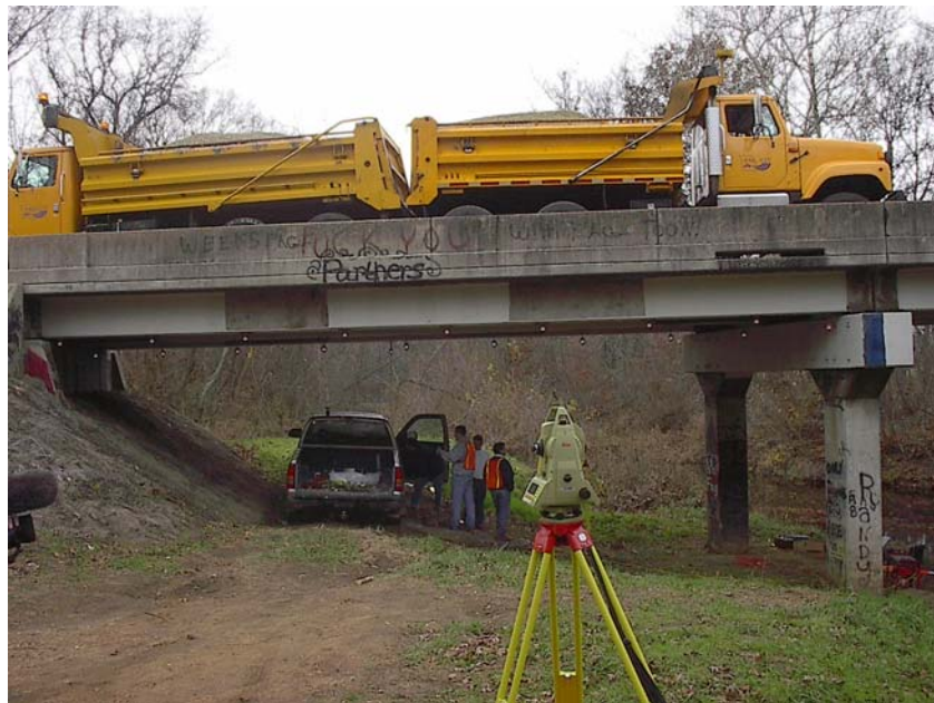
Figure 4.1. Loaded Trucks Used to Test a Bridge
