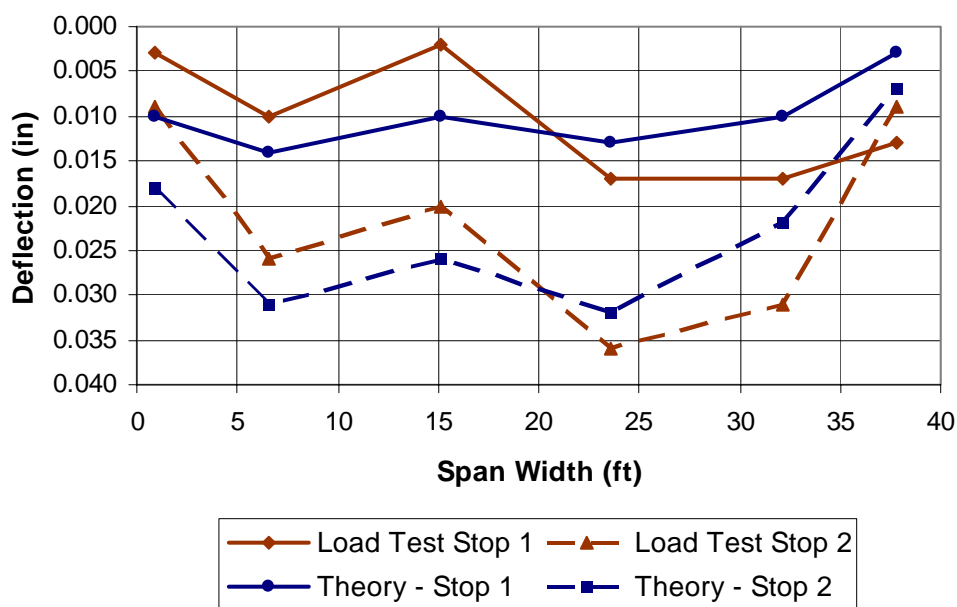
Figure 7.11. Bridge Y-298 East Span
