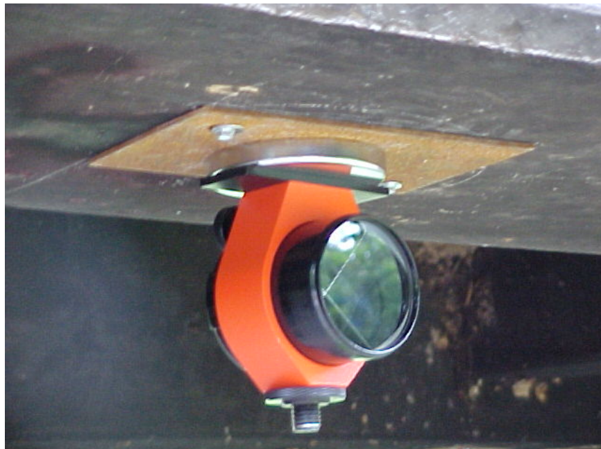
Figure C.3. Short Magnet Mount and Prism
