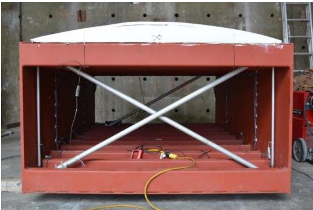
(b) Photograph of the 1/9 th scale tunnel specimen (cross-sectional view)
