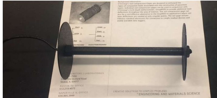
Figure 19. Image of soil compression gauges utilized in test sections
