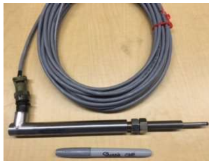
Figure 17. Picture of a Macro Sensor GHS 750-100 LVDT
