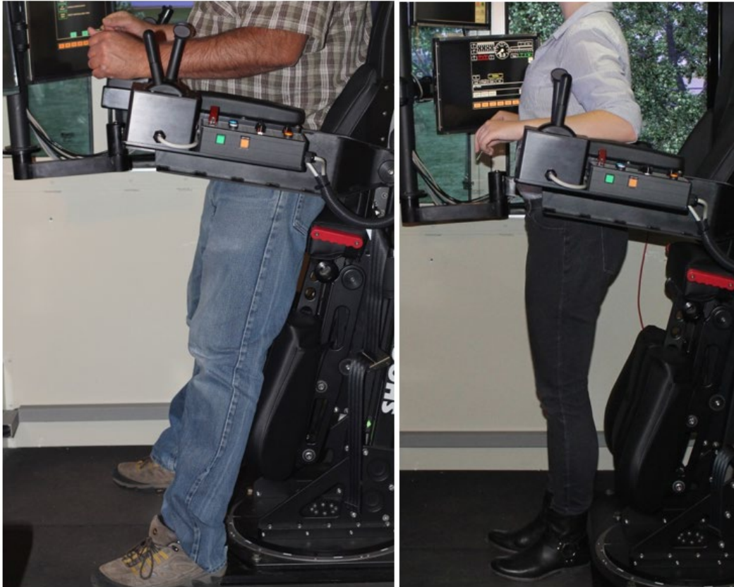
Figure 27. An approximately 95 th percentile male (left) and 50 th percentile female (right) during standing operation demonstrate the lack of armrest adjustability
