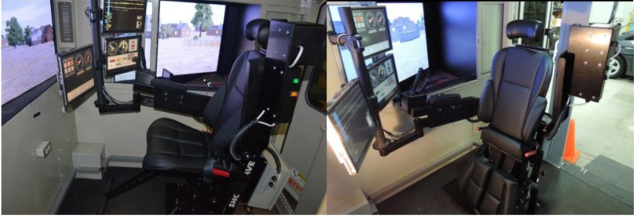
Figure 6. Experimental crewstation configured for seated operation (left) and standing operation (right)
