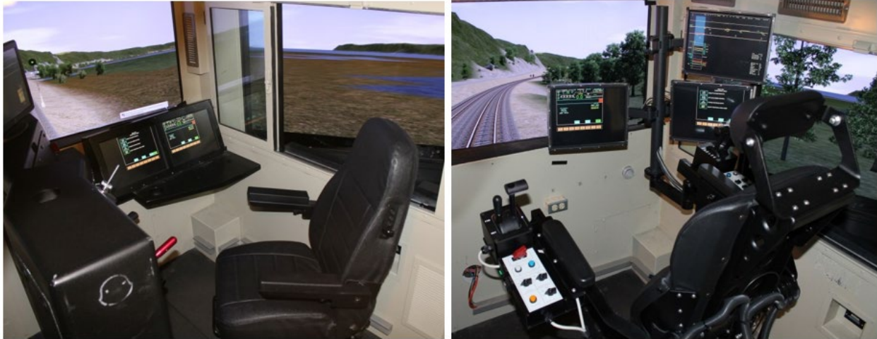
Figure 20. AAR-105 control stand with seat oriented toward controls (left); experimental crewstation with seat and integrated controls oriented toward the front window (right)
