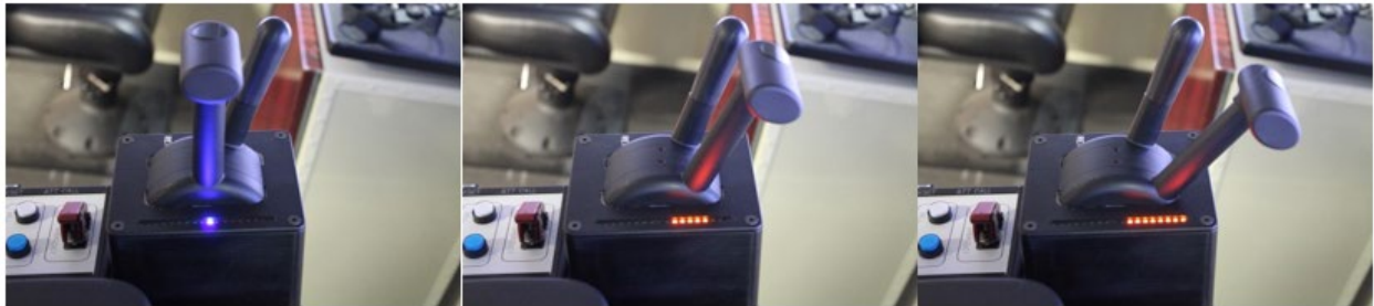
Figure 29. Combined throttle and dynamic brake in a series of positions: set up (left), dynamic notch 5 (center), and dynamic notch 8 (right)
