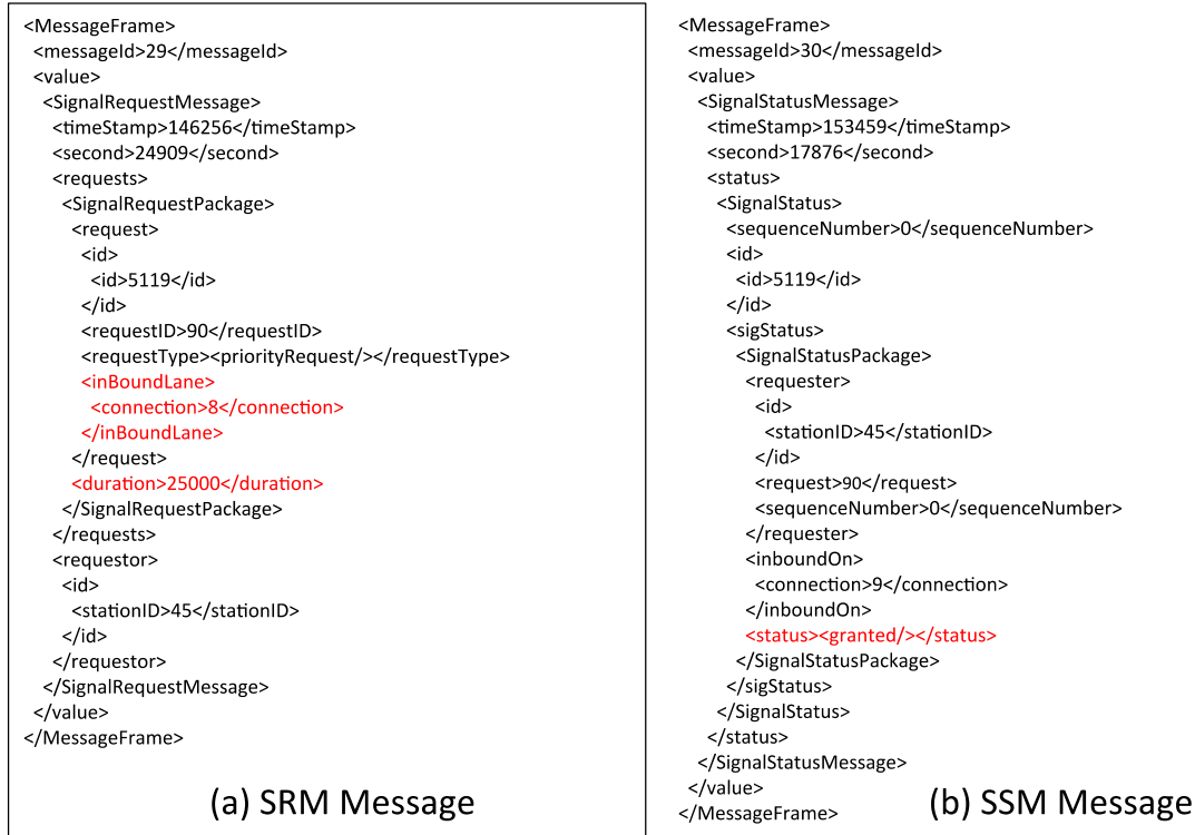
Figure 3-12: Schema for SRM and SSM Message Types
