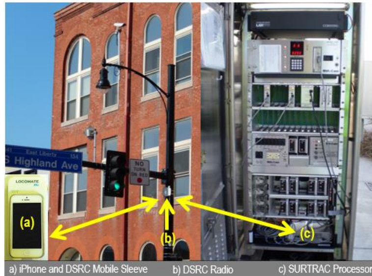
Figure 2-1: Elements of the Safe Intersection Crossing System
