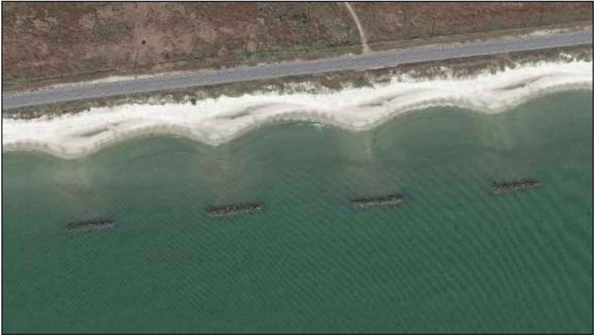
Figure 5-5. Offshore segmented breakwaters and beach nourishment protecting Louisiana Highway 82 in Holly Beach (source: FHWA 2019a).
