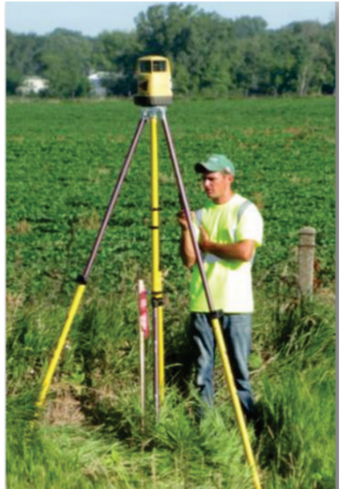
Figure 6. Rotating Laser for controlling elevation (ACPA 2013). © 2013 ACPA
