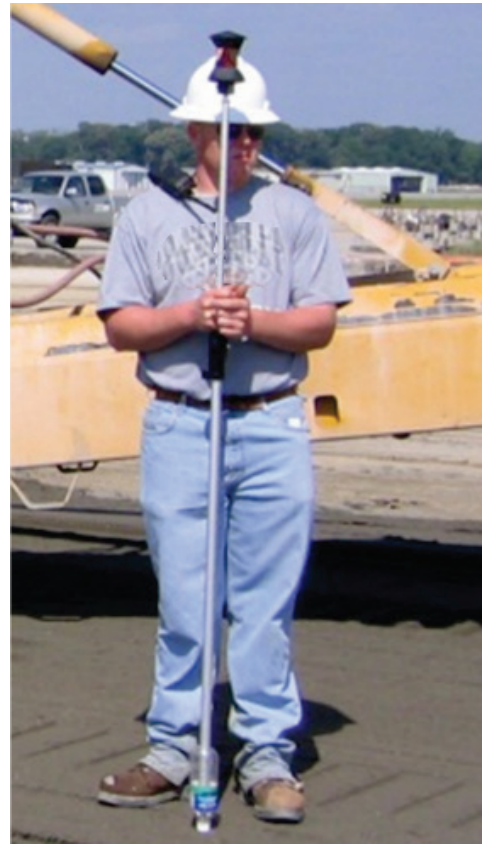
Figure 7. Rover pole for as-built checking (ACPA 2013). © 2013 ACPA
