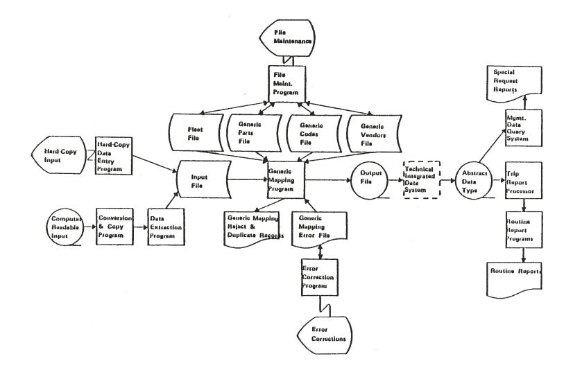
Figure 8. Simplified Bus TRIP EDB system flow diagram.
