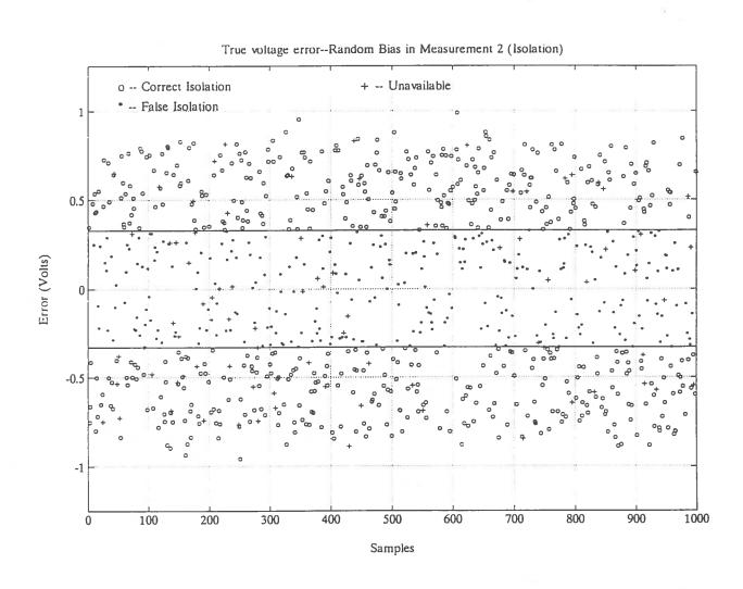
Figure 16 True Voltage Error - Isolation (Bias in Voltmeter 2).
