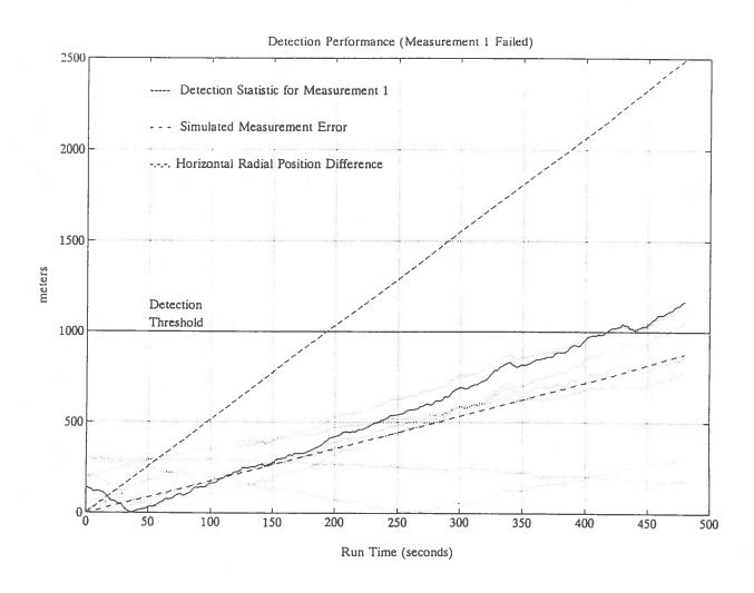
Figure 28 Detection Performance (5 m/s Ramp Error in Measurement 1).
