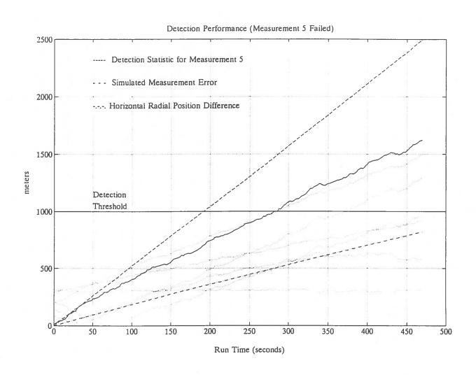
Figure 32 Detection Performance (5 m/s Ramp Error in Measurement 5).
