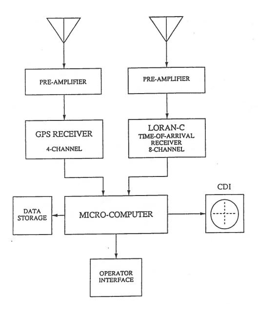
Figure 24 Hardware Configuration of the Prototype Hybrid GPS/Loran-C Receiver.
