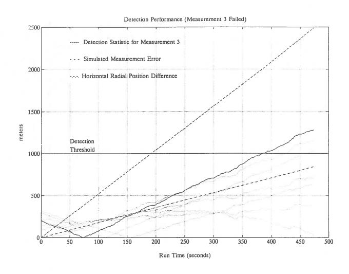
Figure 30 Detection Performance (5 m/s Ramp Error in Measurement 3).
