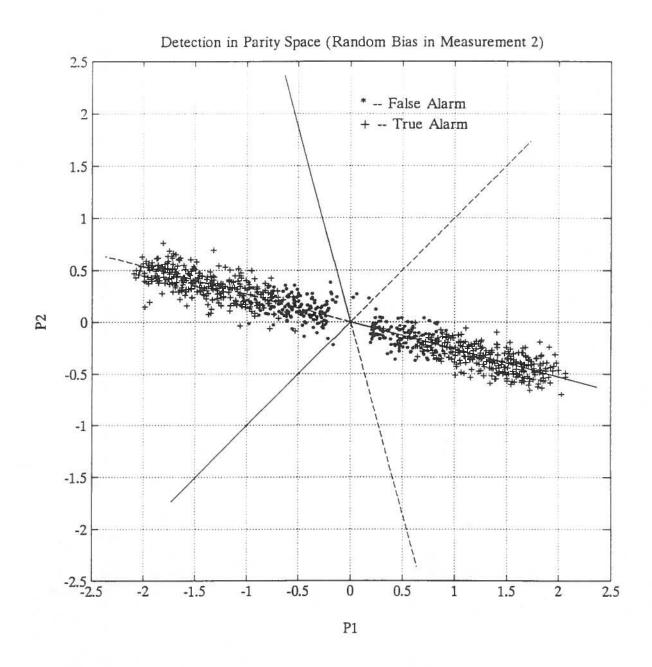
Figure 15 Detection in Parity Space (Bias in Voltmeter 2).
