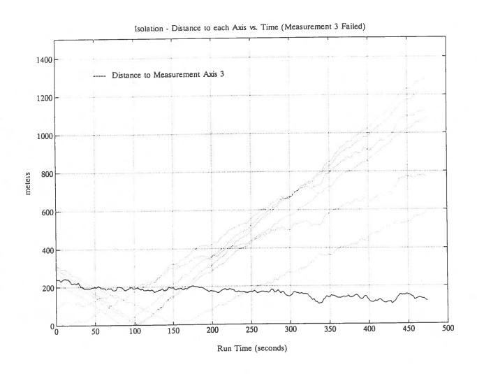
Figure 40 Isolation Performance (5 m/s Ramp Error in Measurement 3).
