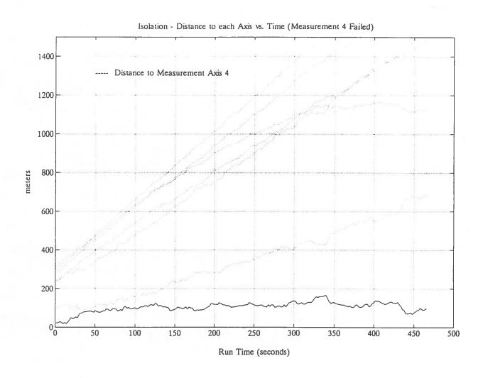
Figure 41 Isolation Performance (5 m/s Ramp Error in Measurement 4).
