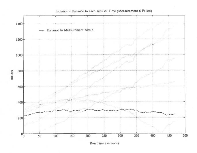
Figure 43 Isolation Performance (5 m/s Ramp Error in Measurement 6).
