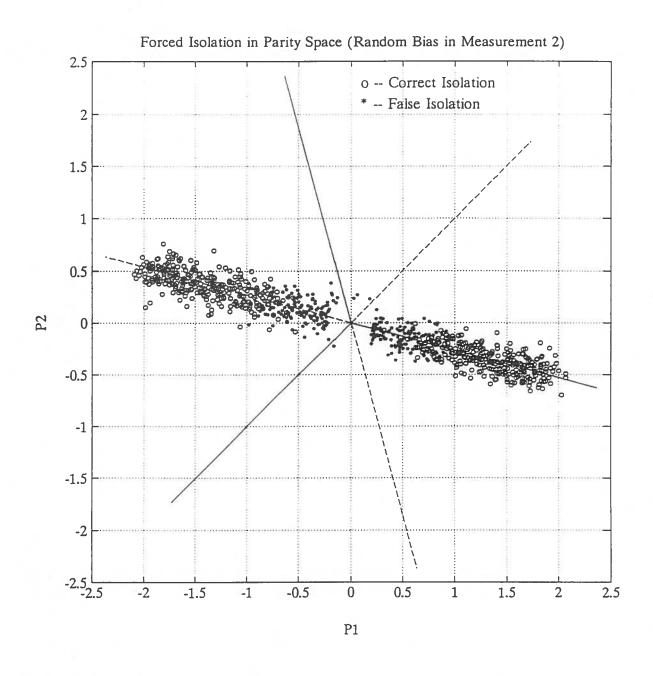
Figure 18 Forced Isolation in Parity Space (Bias in Voltmeter 2).
