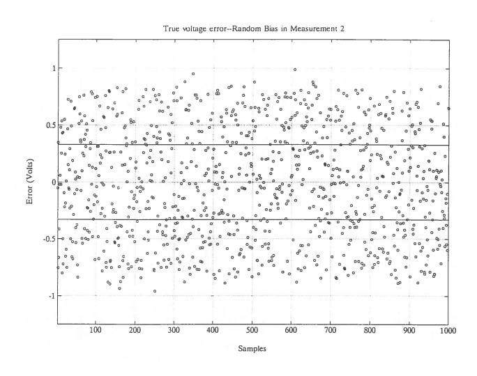
Figure 12 True Voltage Error (Bias in Voltmeter 2).
