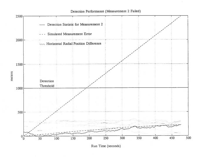
Figure 29 Detection Performance (5 m/s Ramp Error in Measurement 2).
