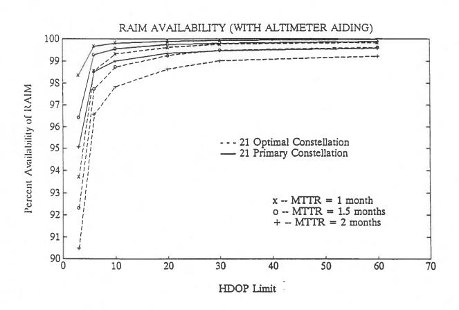
Figure 21 Availability of Fault Detection with Altimeter Aiding.
