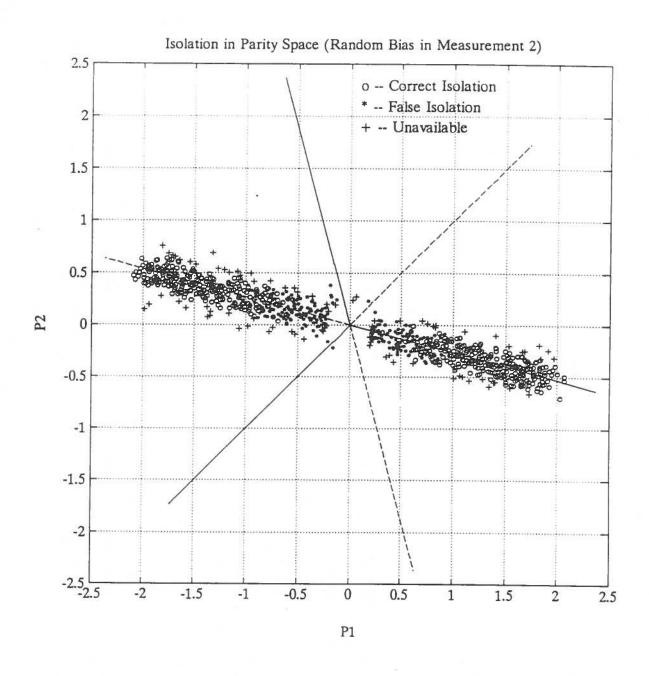
Figure 17 Isolation in Parity Space (Bias in Voltmeter 2).
