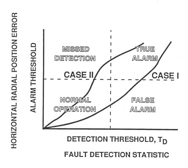
Figure 1 Example of the Impact of Slowly Growing Measurement Errors on Fault Detection.
