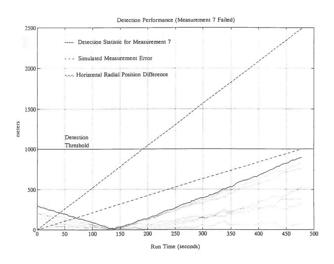
Figure 34 Detection Performance (5 m/s Ramp Error in Measurement 7).
