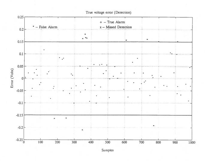
Figure 7 True Voltage Error - Detection (No Bias).
