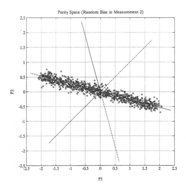
Figure 14 Measurement Points in Parity Space (Bias in Voltmeter 2).
