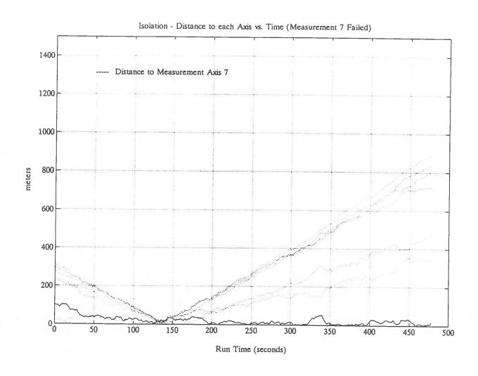
Figure 44 Isolation Performance (5 m/s Ramp Error in Measurement 7).
