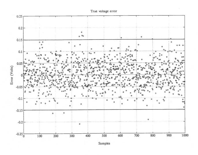
Figure 6 True Voltage Error for 1000 Samples (No Bias).
