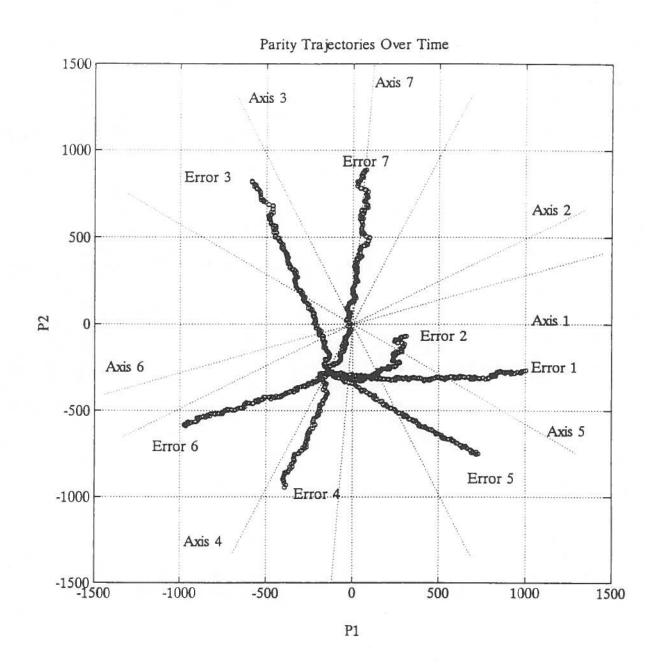
Figure 35 Trajectories of the Parity Vectors over Time for all 7 Simulated Measurement Errors.
