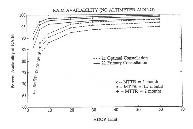
Figure 20 Availability of Fault Detection without Altimeter Aiding.
