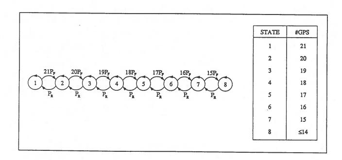
Figure 19 Markov Diagram for GPS (21 Satellites).
