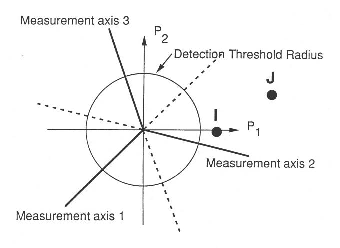
Figure 4 Example of Isolation Problem for Three Voltmeters.
