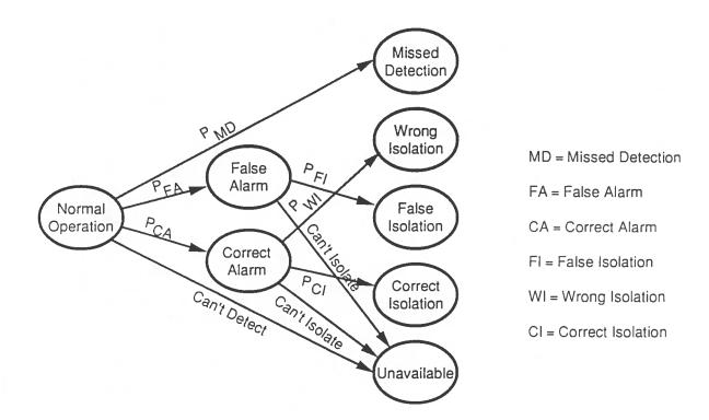
Figure 5 Fault Detection and Isolation State Diagram.
