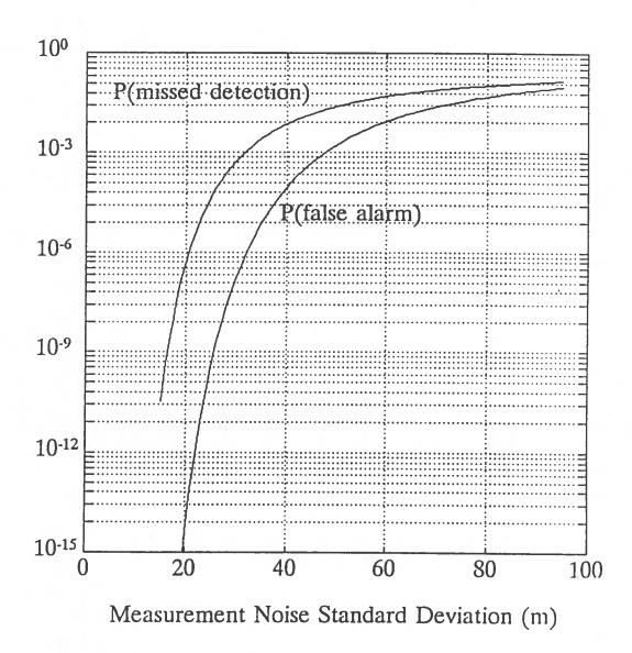
Figure 22  $P_{FA}$  and  $P_{MD}$  as a Function of Measurement Noise ( $T_D = 157$  meters).
