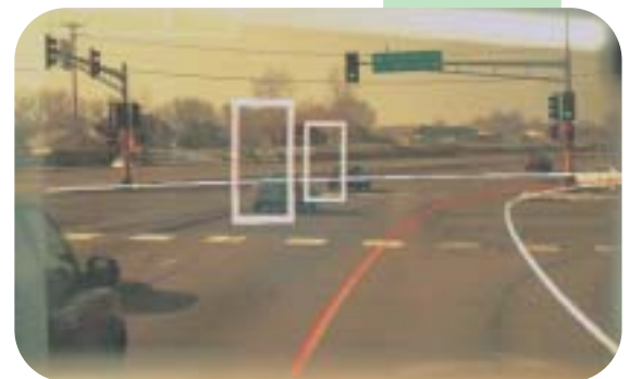
Vehicle-lane assist technology generates projected travel path for the transit bus.
