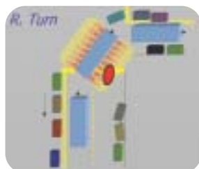
Schematic representation of ultrasonic sensors detecting objects on the sides of a right-turning bus.
