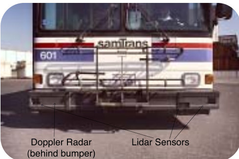
Front view of a San Mateo County Transit District bus equipped with the frontal collision warning system.
