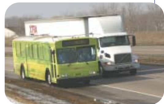
A Metro Transit bus, equipped with the vehicle-lane assist technology, driving on bus-only shoulder.
