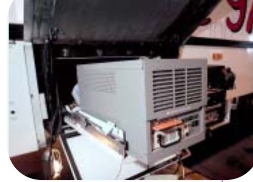
Frontal collision warning system software runs on a standard Pentium computer accessible via a door in the side of the bus. (Prototype shown in this photo.)
