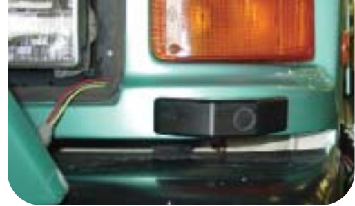
Corner sensor installed on a Port Authority of Allegheny County bus.
