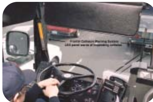
Interior view of a San Mateo County Transit District bus equipped with the frontal collision warning system. Driver Vehicle Interface lightbars warn driver of impending collision.
